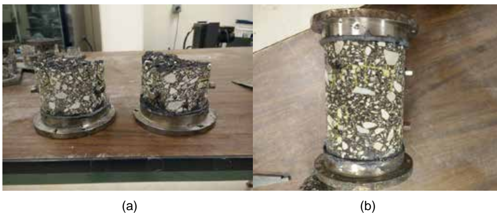
Figure 3.21: (a) Fully-Cracked S-VECD Sample, (b) S-VECD Sample with Micro-Cracks
