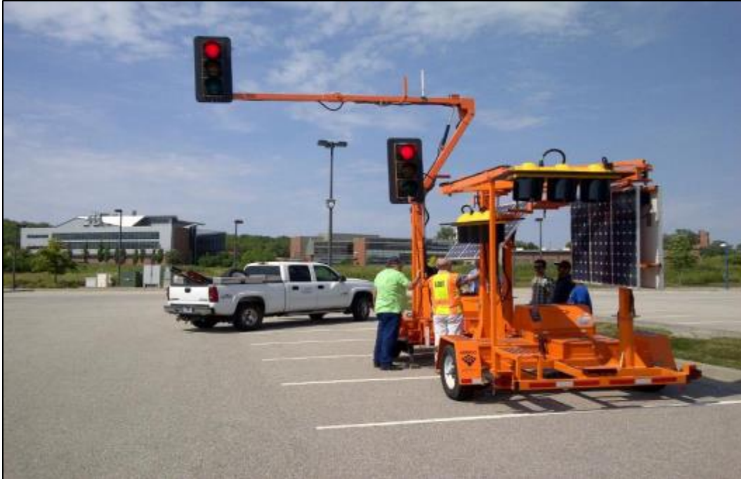
Figure 3.1: Closed-Course Field Testing of the Signal Units at the University of Kansas
