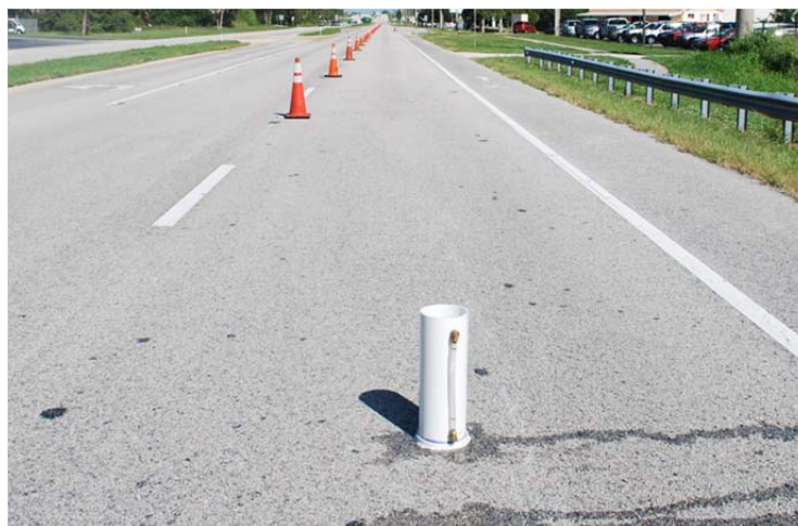
Figure 3-11. Field drainability testing on US-1.
