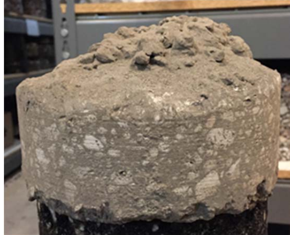
Figure 3-7. OGFC surface layer plus dense-graded under layers specimen after Cantabro loss test.
