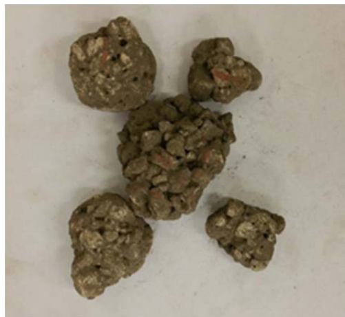
Figure 3-6. OGFC surface layer specimen after Cantabro loss test.
