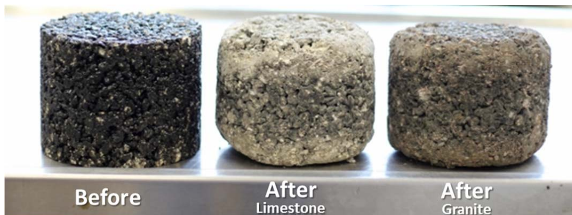
Figure 5-4. Cantabro abrasion loss specimens before and after testing.
