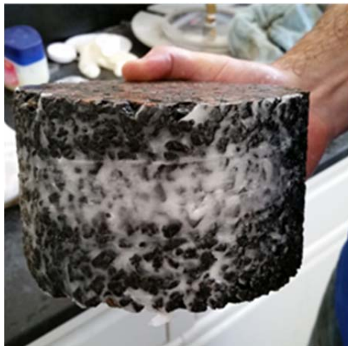
Figure 5-2. Permeability specimen sealed with petroleum jelly.
