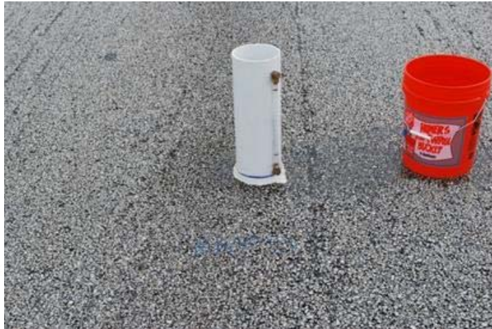
Figure 3-3. Field drainability test: (a) schematic (TxDOT 2009), (b) field setup.
