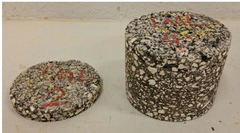
Figure 3-5. Specimens used for Cantabro loss test; OGFC surface layer only (left), OGFC surface layer plus dense-graded under layers (right).
