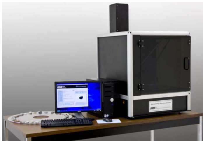
Figure 4-2. Second-generation Aggregate Image Measurement System—AIMS2 (Gates et al. 2011).
