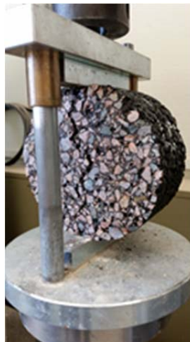
Figure 5-6. Laboratory specimen from mixture 6 after IDT strength test failure.
