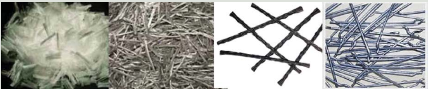
Figure 1 Polypropylene fibrillated fiber (left), polypropylene macro fiber (left middle), carbon fiber (right middle) and steel fiber (right)
