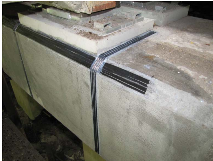
Figure 18 Detail of horizontal and vertical tows junction
