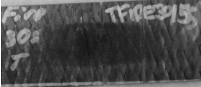
Figure 8: Fibers exposed due to fire damage
