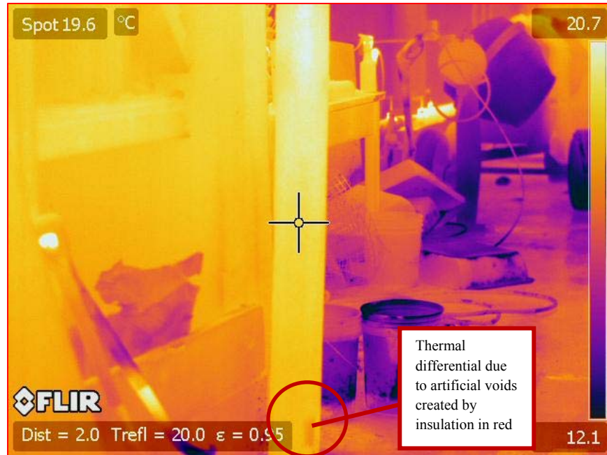
Figure 20: Partially filled Tube K, 12:24, time since filling ~30 minutes
