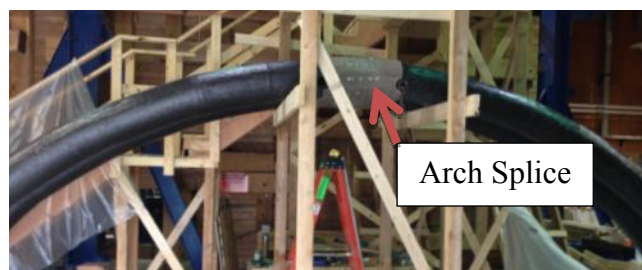
Figure 12: Key inspection location, spliced arch in laboratory
