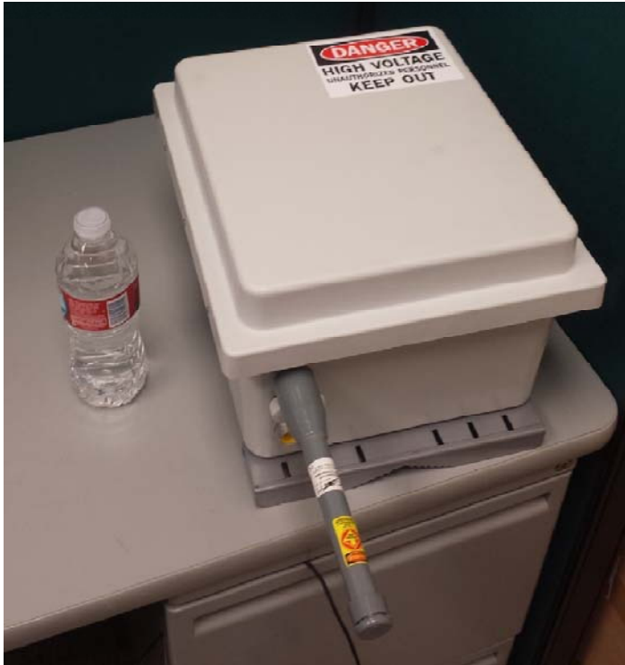
Figure 6 Bluetooth probe detection system cabinet
