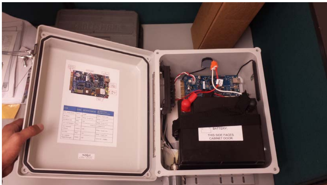
Figure 7 Components of Bluetooth probe detection system
