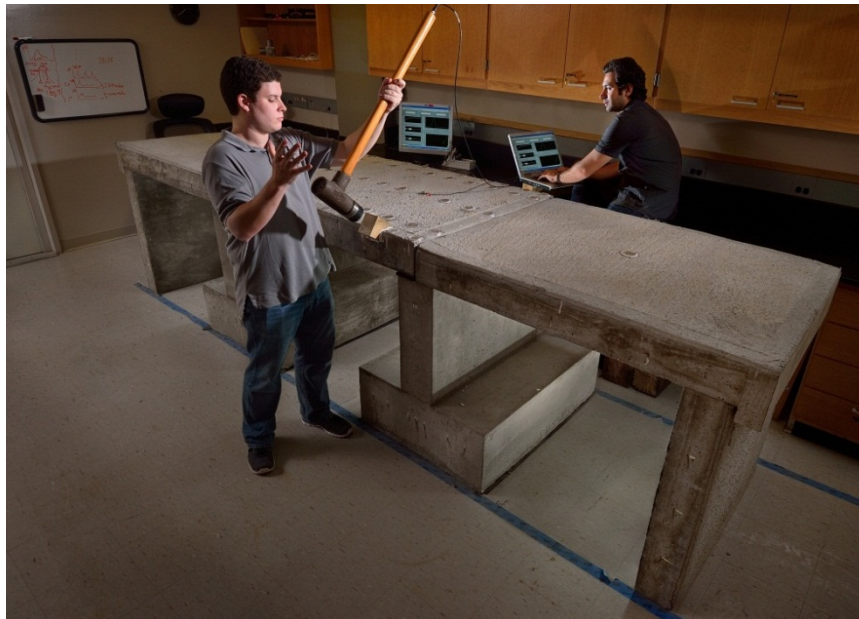
Figure 2. Impact hammer testing with Steven Worley and labmate Farhad Sedaghati.
