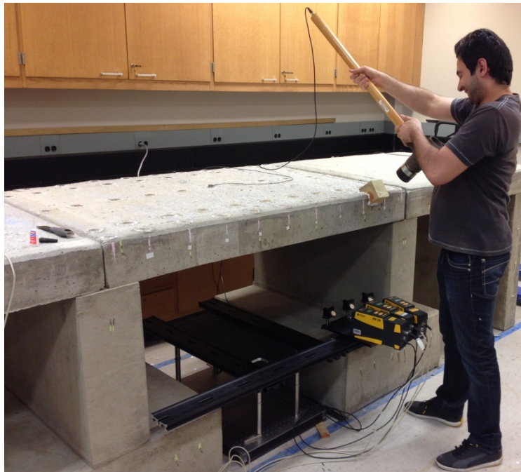
Figure 10. Impact test in progress.
