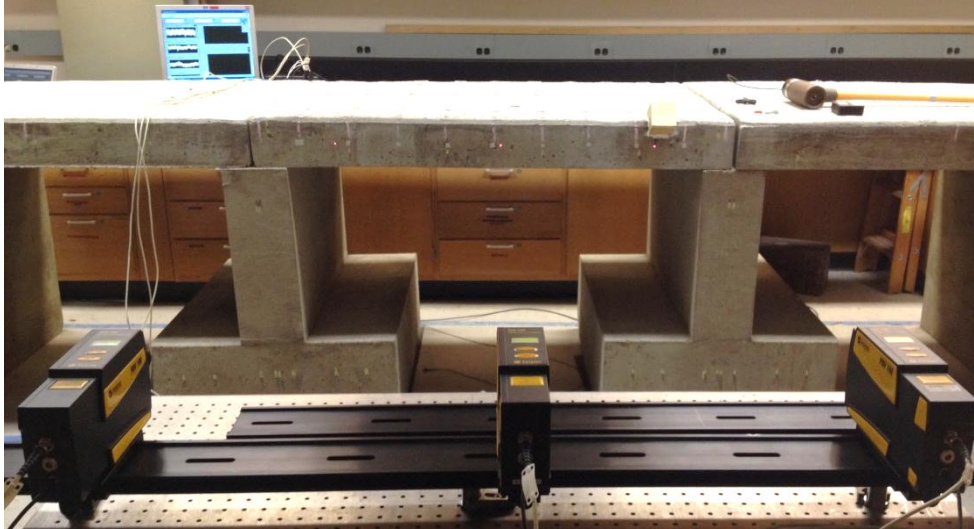
Figure 3. Preliminary test setup with three LDVs shooting target slab vibrations.
