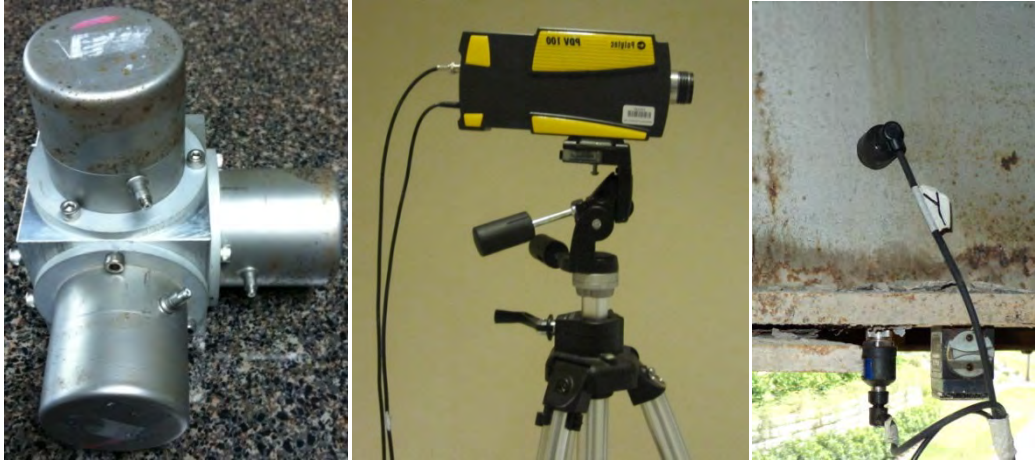
Figure 31. Tri-axial accelerometer (left), laser Doppler vibrometer (middle), and magnetic accelerometers and corner cube reflector array (right).
