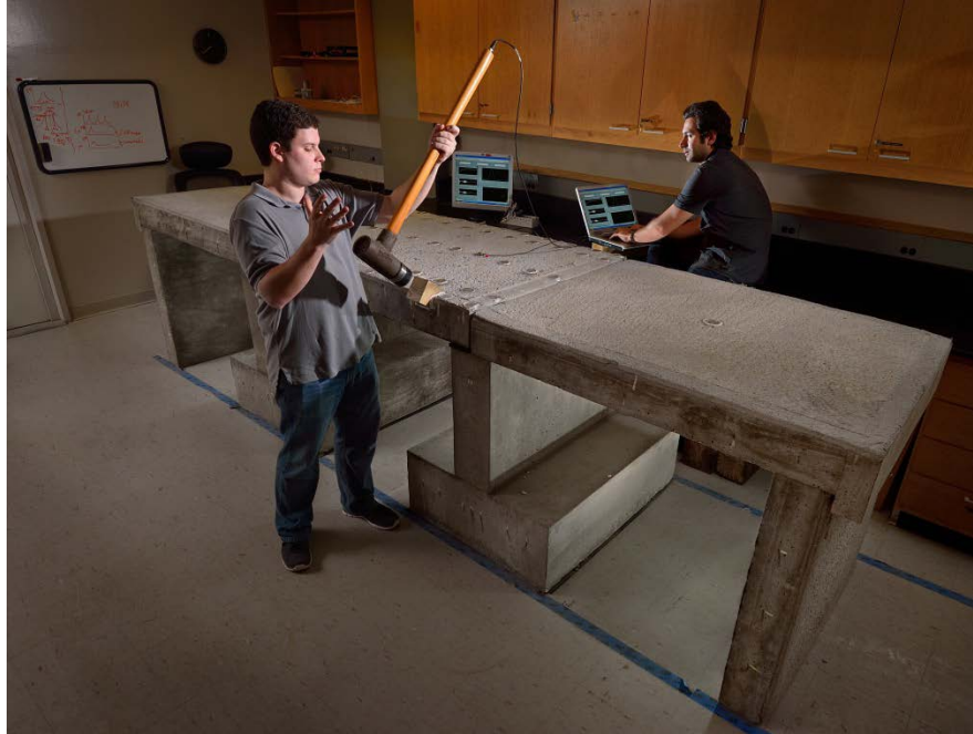
Figure 25. Impact hammer testing with Steven Worley and labmate Farhad Sedaghati.
