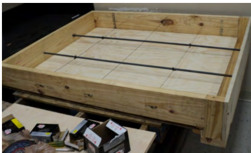
Figure 14. The first of two end slab forms. Figure 15. The second of two center slab forms.
