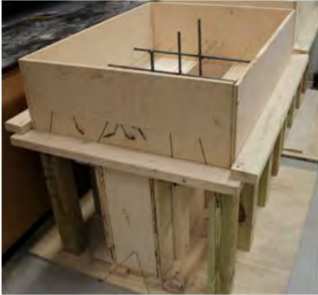
Figure 16. The first of two t-shaped pier forms. Figure 17. The second of two end wall forms.
