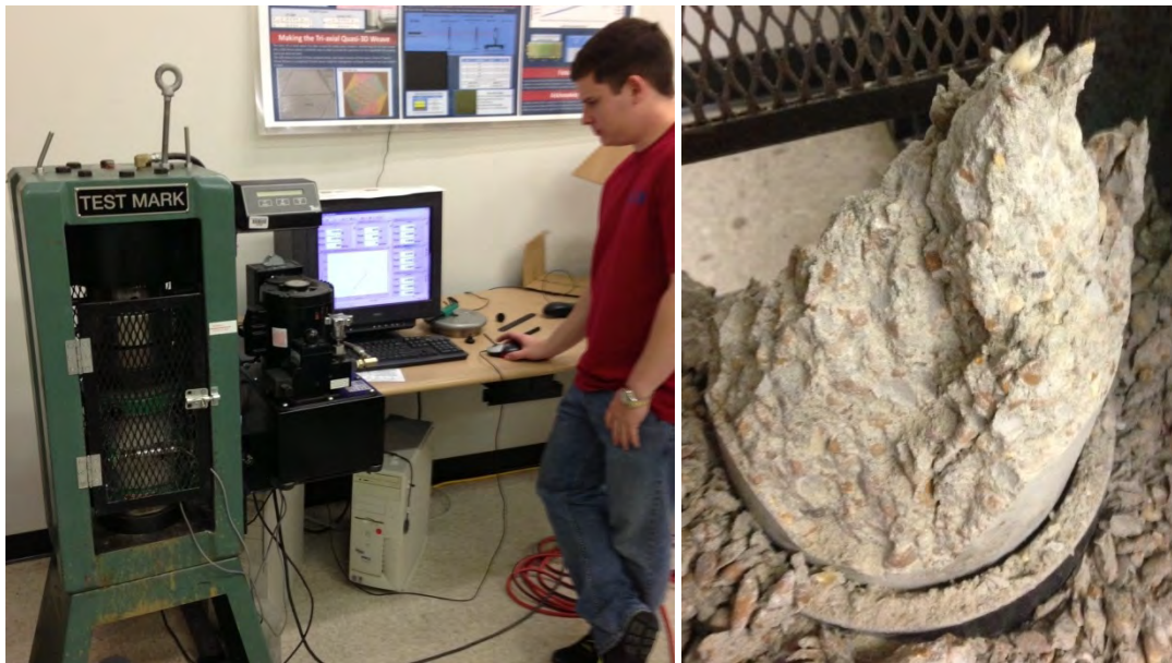
Figure 22. Testing of a cylinder and the resulting break.
