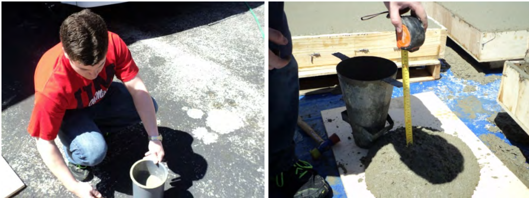
Figure 21. Cylinder casting and slump test.
