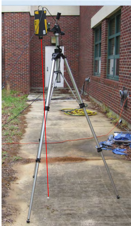
Figure 8. Setup for measuring LDV tripod response.
