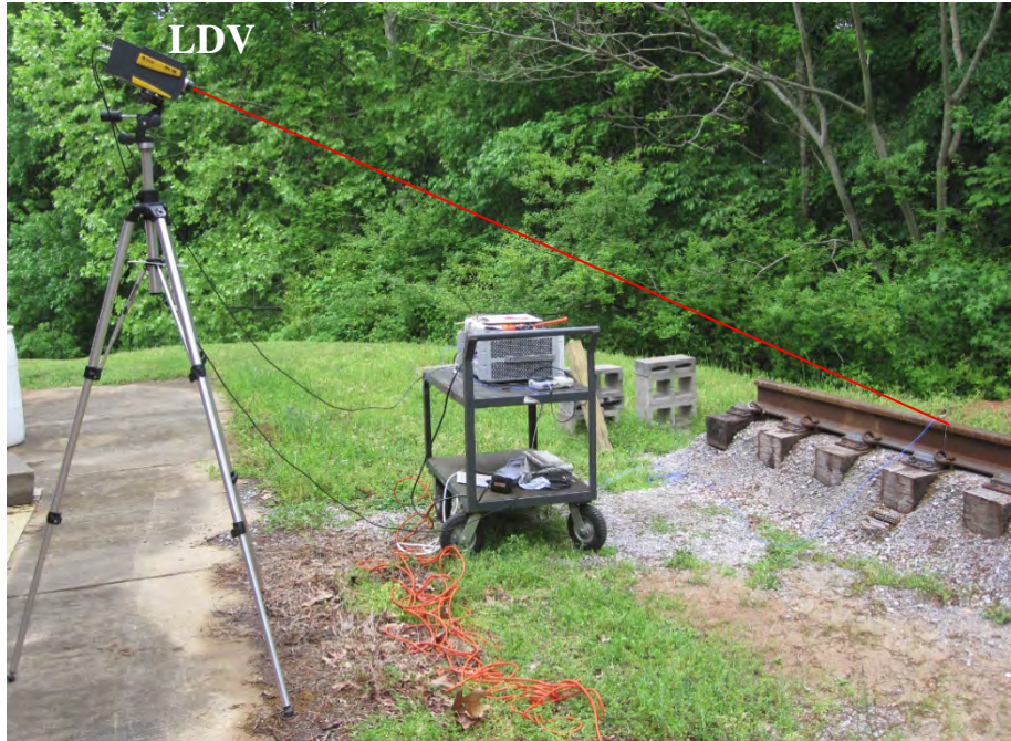
Figure 5. Photograph of the instrumented rail experiment for LDV sensitivity.
