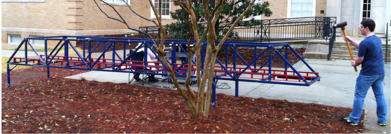
Figure 38. Testing in progress on the student-ASCE cantilever steel truss. Baseline shown.
