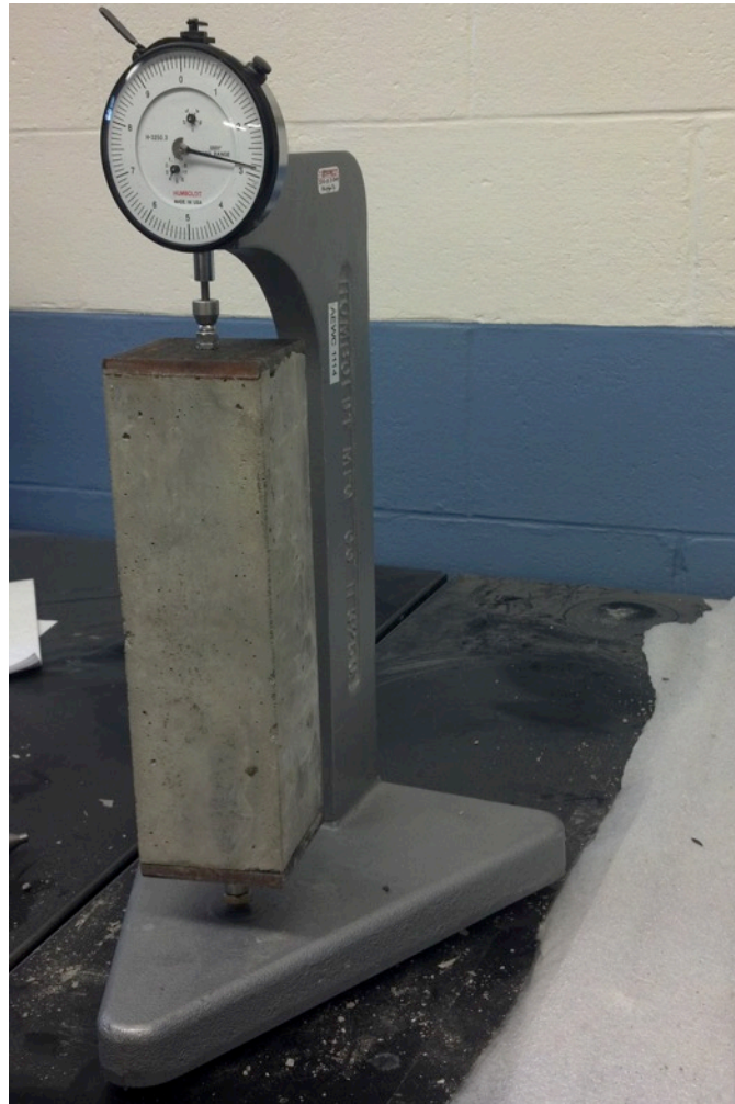
Figure 5 – Expansion Specimen Measurement in Comparator
