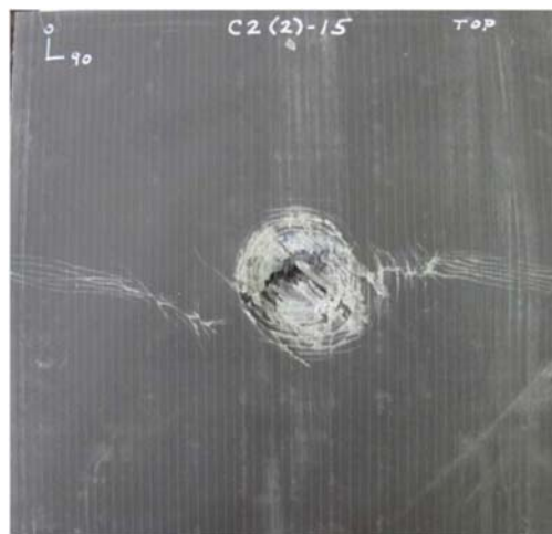
Figure 9: Cracks form around a puncture (Kittridge et al [5])
