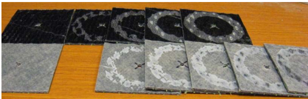
Figure 3: Discoloration due to abrasion, study samples
