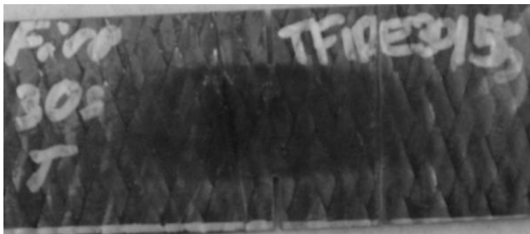
Figure 7: Fibers exposed due to fire damage
