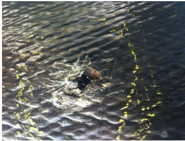
Figure 4: Full puncture/hole in carbon fiber laminate
