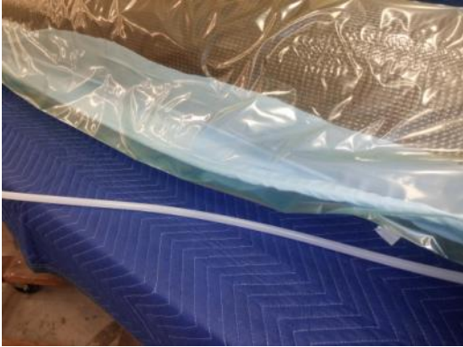
Figure 5: Bagging film ridges acceptable in the resin layer of a BiaB FRP tube
