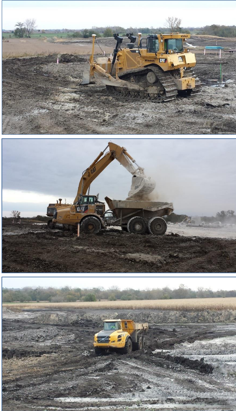
Figure 2. Equipment monitored on site: CAT D8T bulldozer (top), CAT 375 Hydraulic Excavator and CAT 740 B truck (center), and Volvo A40F truck (bottom)
