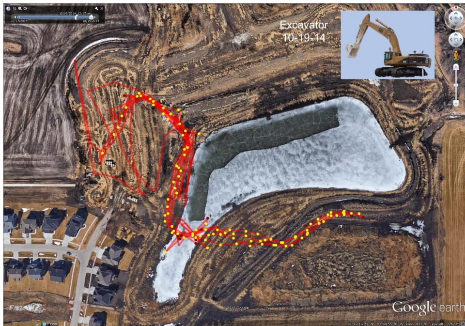
Figure 21. CAT 375 excavator operations for October 19
