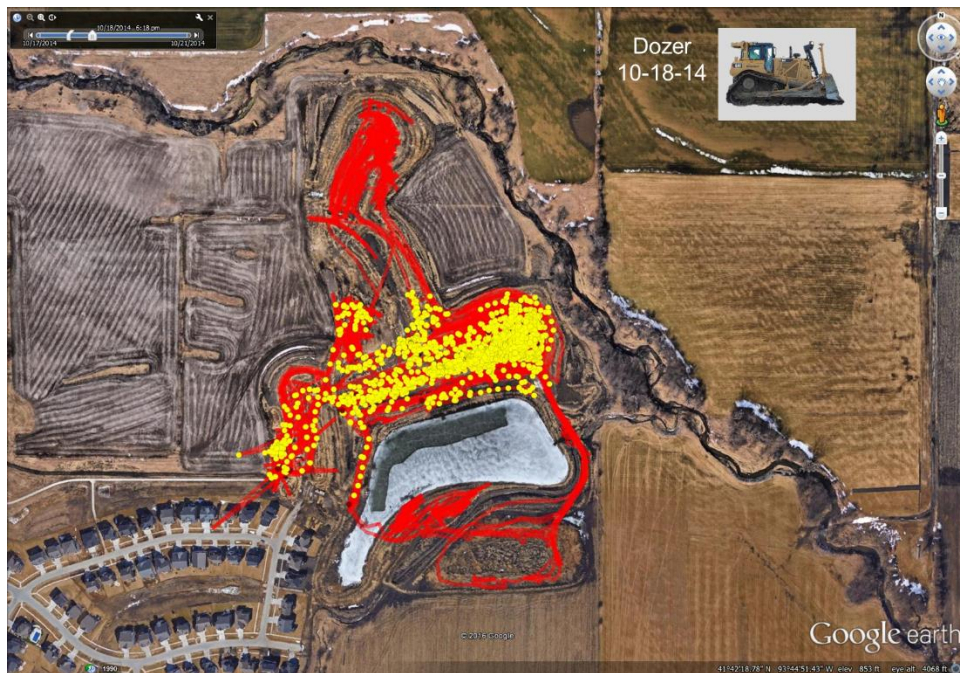
Figure 14. CAT D8T bulldozer operations for October 18
