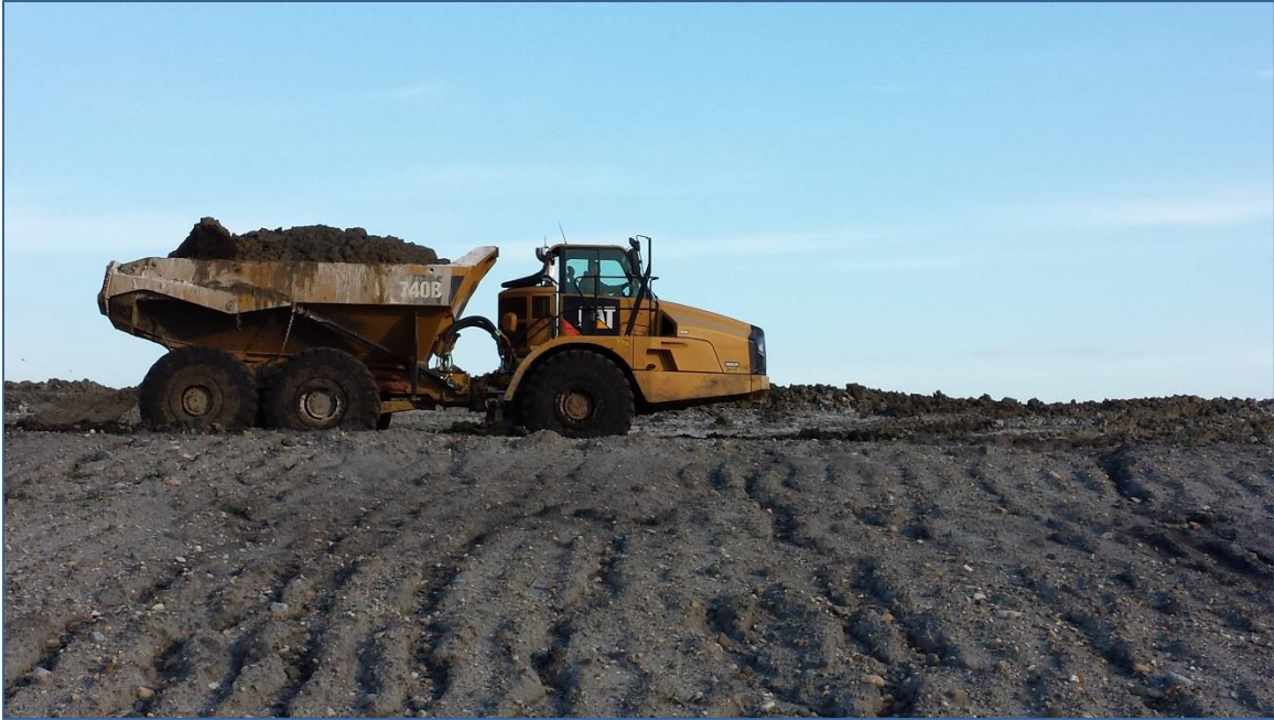
Figure 9. Loaded CAT 740B haul truck traveling on haul road to fill area
