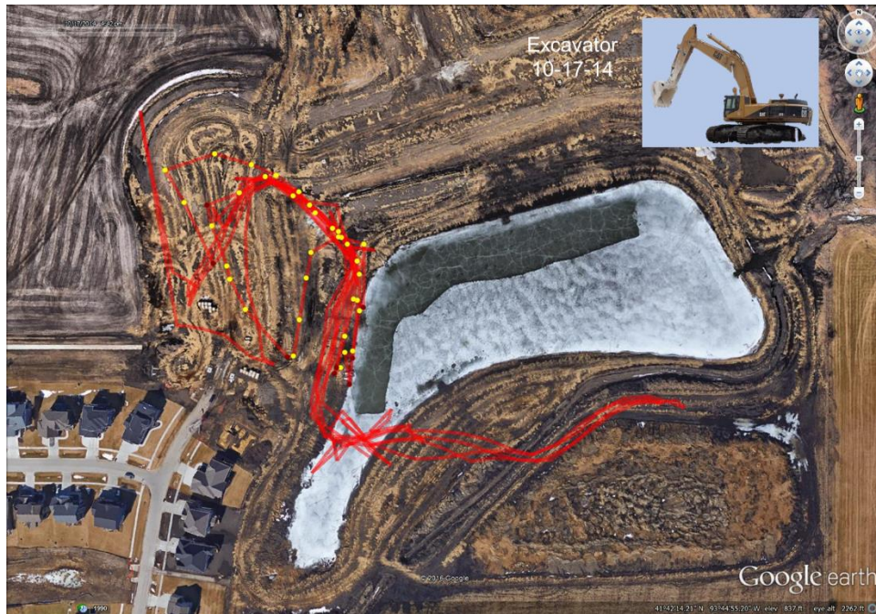
Figure 19. CAT 375 excavator operations for October 17
