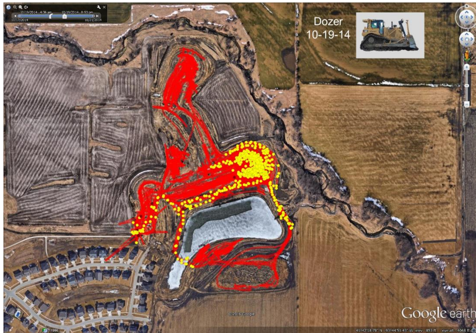
Figure 15. CAT D8T bulldozer operations for October 19
