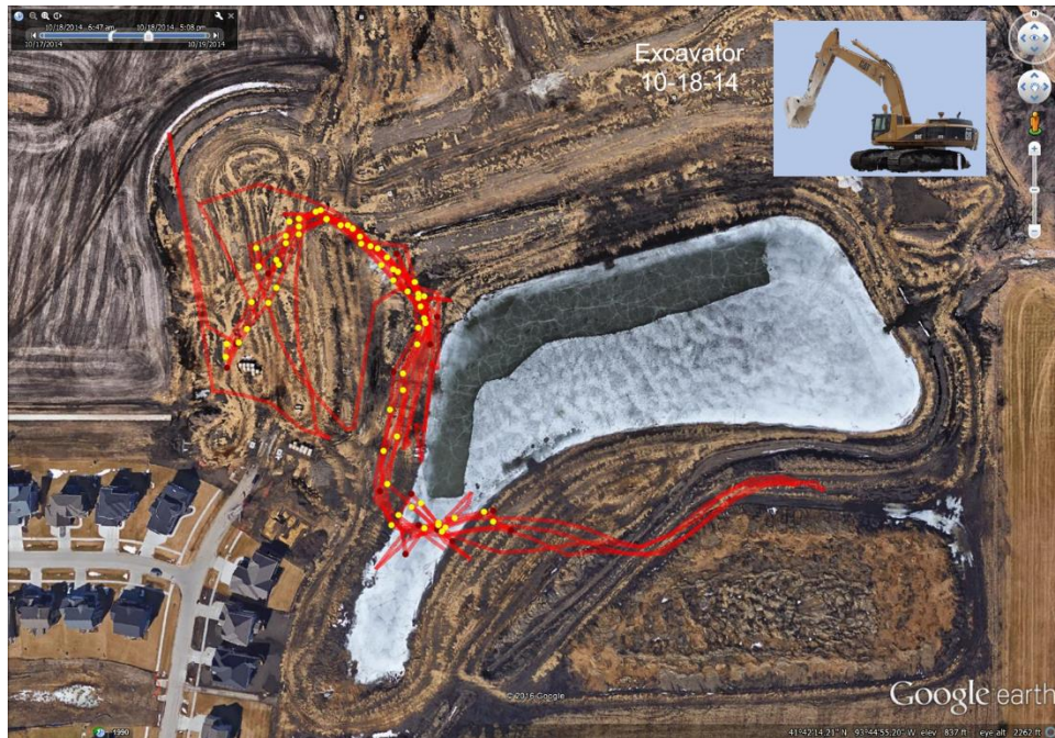
Figure 20. CAT 375 excavator operations for October 18
