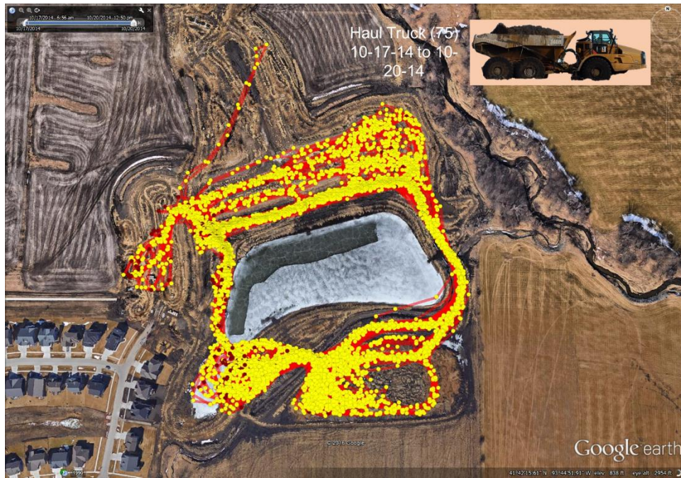
Figure 22. CAT 740B haul truck (#70075) operations for October 17 through October 20
