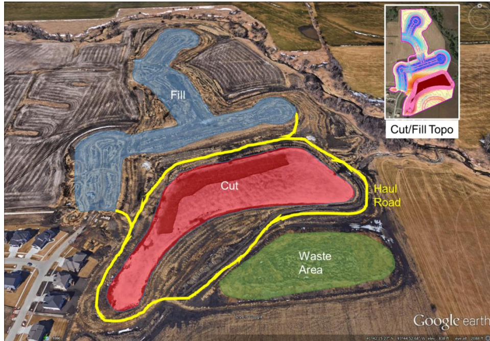
Figure 1. Idealized cut/fill/haul details for the project
