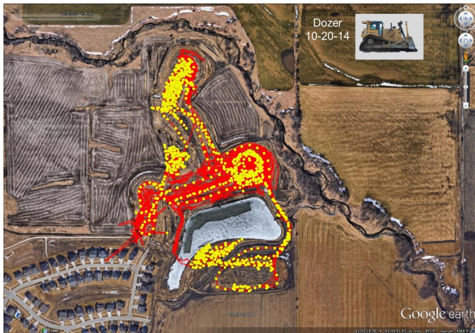
Figure 16. CAT D8T bulldozer operations for October 20
