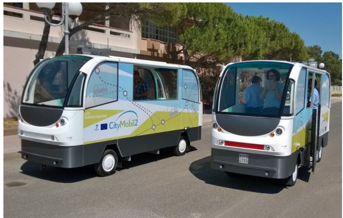
Figure 11. The CityMobil2 buses can hold up to eight people at once and are narrower than even most small European cars.
