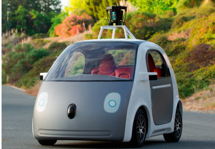
Figure 17. Highly autonomous L5 car designed by Google to function solely as a passenger vehicle.
