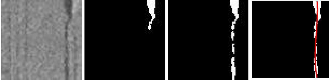
Figure 13. Example of polynomial fitting of noncontinuous crack (left to right): raw crack block, maximum extraction, maximum expansion, and polynomial fitting
