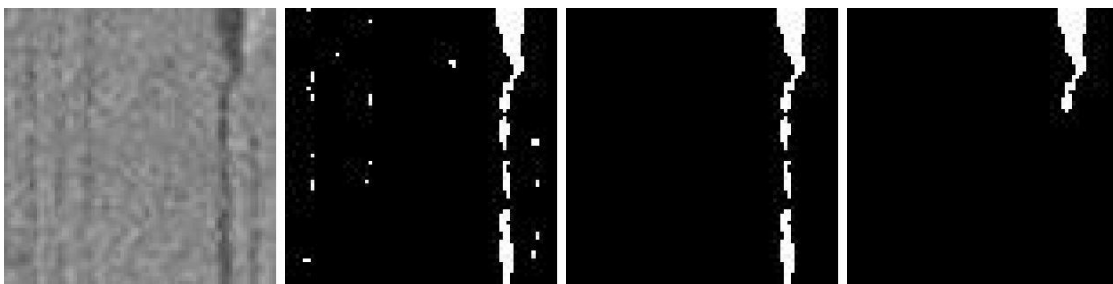
Figure 7. Example of noncontinuous pavement crack at medium severity (from left to right): raw crack block, local filtering, minor removal, and maximum extraction
