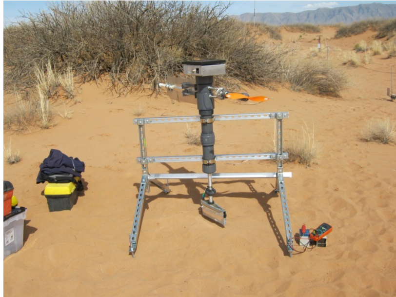
Figure 1. Photograph of prototype sand movement sensor platform developed under NSF funding and deployed for field testing at the Jornada experimental range in New Mexico.
