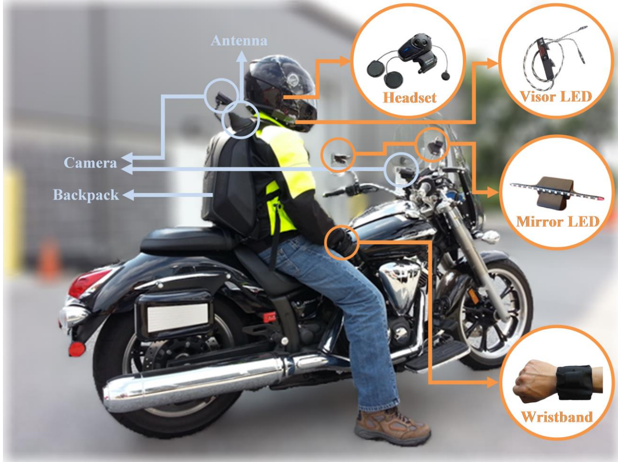
Figure 1. A rider on a Yamaha V Star with a connected motorcycle CWS.
