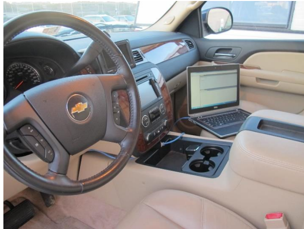
Figure 5. The in-vehicle computer and its control interface.
