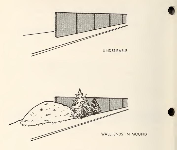
FIGURE 3-23. USE OF EARTH MOUND TO TERMINATE WALL
