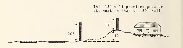
FIGURE 3-4 Use of Elevated Terrain to Achieve Greater Attenuation with Lower Walls.
