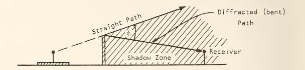
FIGURE 2-2 Barrier Diffraction.
