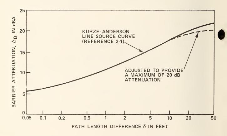
FIGURE 2-4 BARRIER ATTENUATION FOR A LINE OF INCOHERENT POINT SOURCES.
