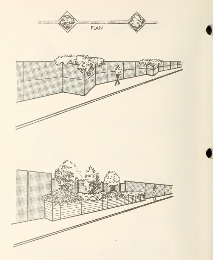
FIGURE 3-16. USE OF LANDSCAPING TO IMPROVE BARRIER APPEARANCE and color should be explored, as shown in Figure 3-17. In other areas, particularly those closely related to freeway structures or other transportation elements, it becomes desirable that the barriers have a strong visual relationship, either physically or by design concept, to the highway elements. See Figure 3-18 for an example.
