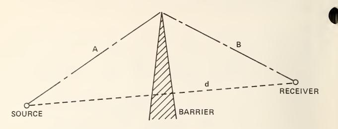
FIGURE 2-3 ILLUSTRATION OF PATH LENGTH DIFFERENCE.
