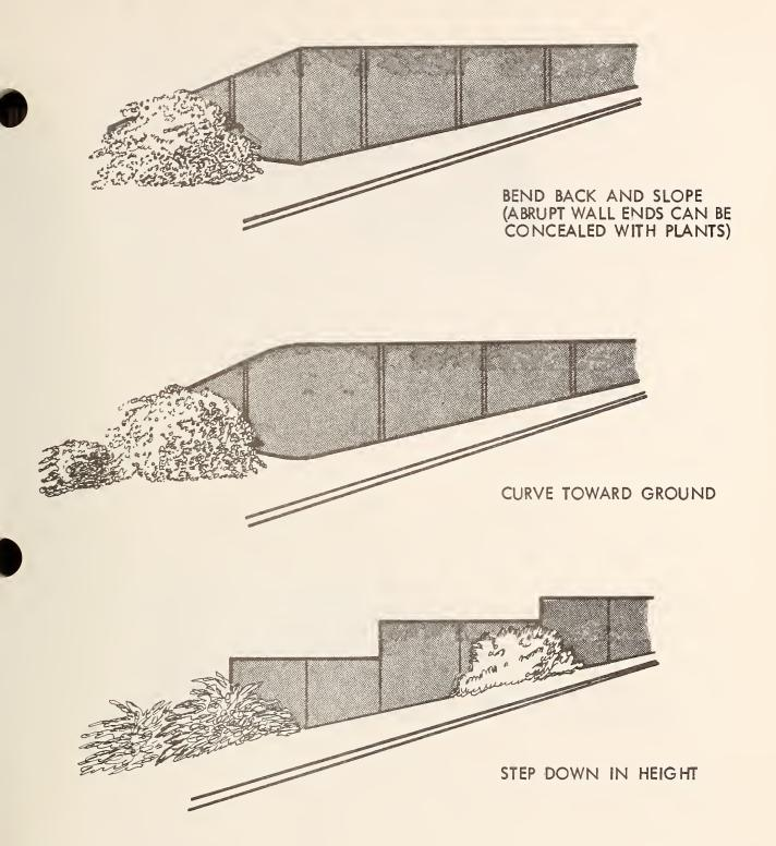
FIGURE 3-24. ALTERNATE MEANS OF TERMINATING BARRIER WALLS
