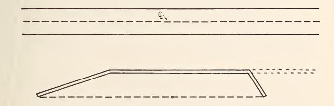
FIGURE 3-7 Use of Short Segments Wrapped Around the Receiver to Achieve an "Infinite" Barrier.
