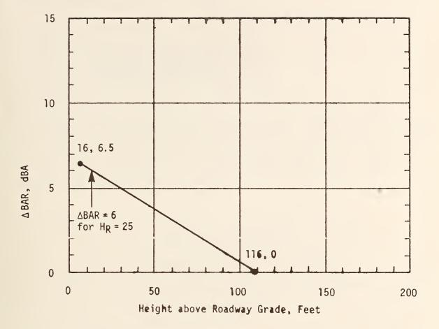
FIGURE 4-23 Use of Grid to Determine  $\triangle BAR$ .
