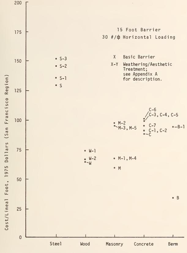
FIGURE 3-30 Construction Costs for Barriers with Additional Treatments.
