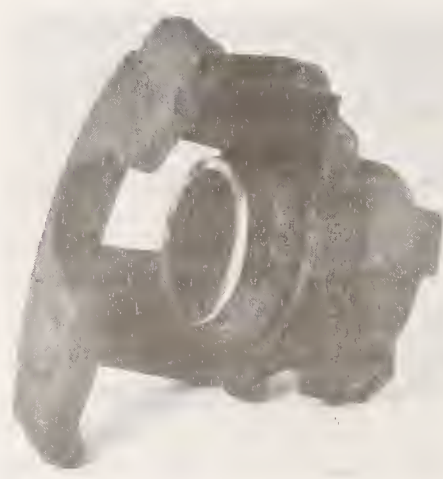
Corroded Pinto Pistons
