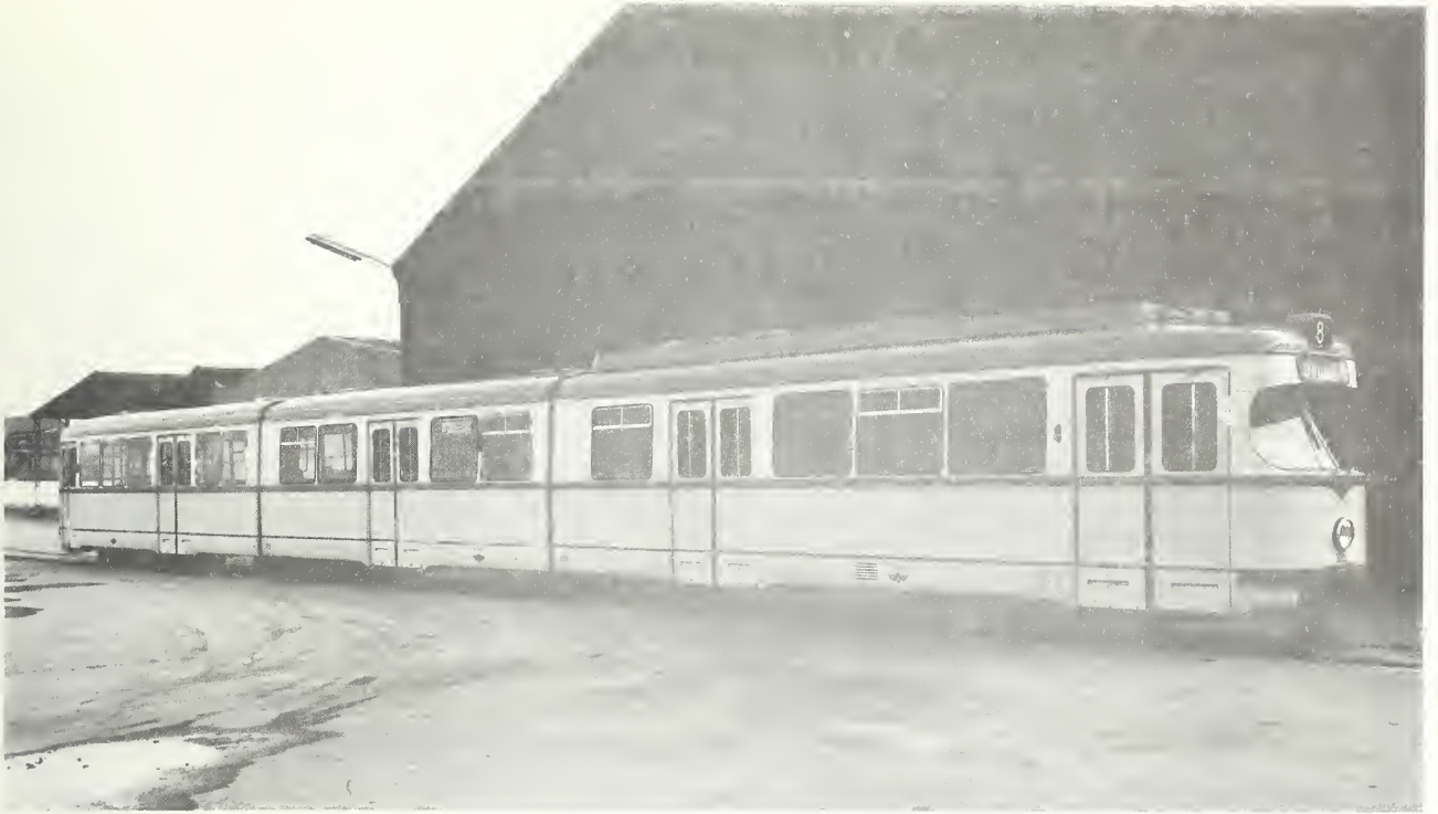
P-7 . Eight-axle double-articulated 2.5 m. (8'2") wide car
