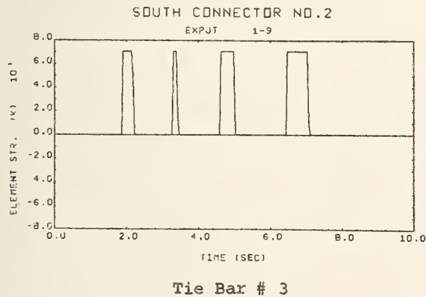
Fig. 43 Longitudinal Tie Bar Forces and the Corresponding Plastic Elongations at Expansion Joint # 1
