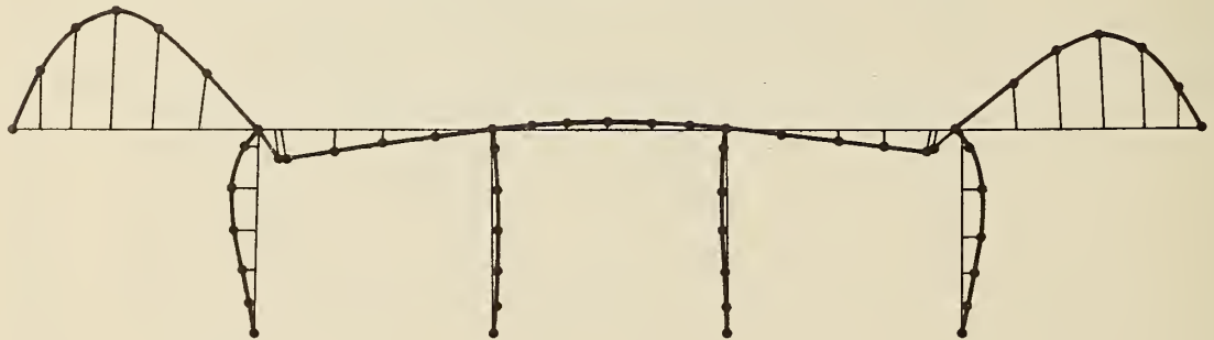
FIG. 5.2.2 CALCULATED LOWEST VIBRATION MODE; TRANSVERSE (Y) DIRECTION
