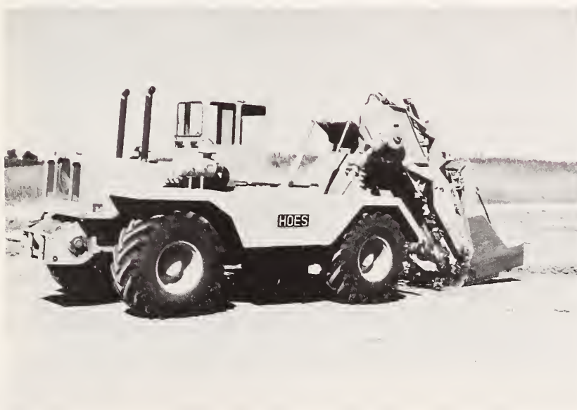
Figure 6.20. High Speed Trenching Machine.
