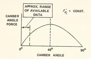
Figure 3.20 ASSUMED VARIATION OF CAMBER FORCE WITH CAMBER ANGLE
