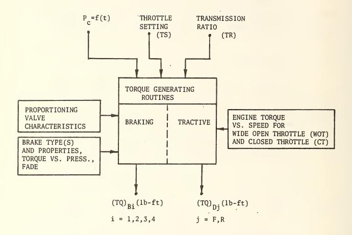
Figure 3.8 GENERATION OF WHEEL TORQUES
