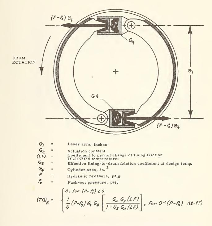
Figure 3.11 TYPE 2 BRAKE - DRUM TYPE WITH TWO LEADING SHOES, TWO CYLINDERS
