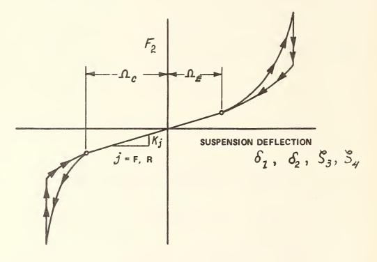
Figure 3.7 GENERAL FORM OF SIMULATED SUSPENSION LOAD-DEFLECTION CHARACTERISTICS (REFERENCE 2)
