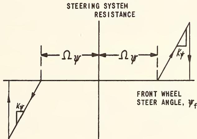
Figure 3.4 STEERING SYSTEM RESISTANCE VS STEER ANGLE
