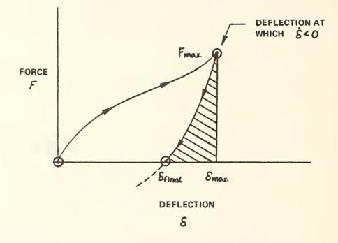
Figure 3.27 GENERAL FORM OF BARRIER LOAD-DEFLECTION CHARACTERISTICS
