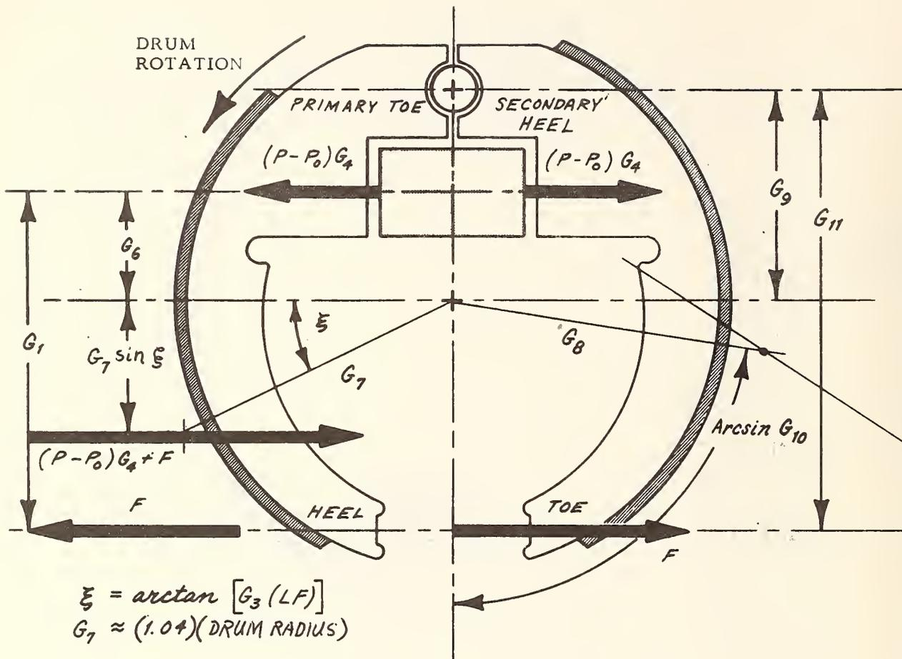
$$(TQ)_B = \begin{cases} 0, & \text{for } (P-P_0) \leq 0 \\ \frac{1}{12} (P-P_0) G_4 \left\{ \left[ 1 + \frac{G_6 + G_7 \sin \xi}{G_1 - G_6 - G_7 \sin \xi} \right] \left[ G_7 \sin \xi + \frac{G_8 G_{11} G_{12} (LF)}{G_9 G_{10} [1 - G_2 G_{12} (LF)]} \right] - \frac{G_1 G_8 G_{12} (LF)}{G_9 G_{10} [1 - G_2 G_{12} (LF)]} \right\}, & \text{for } 0 < (P-P_0) \quad (\text{LB-FT}) \end{cases}$$
