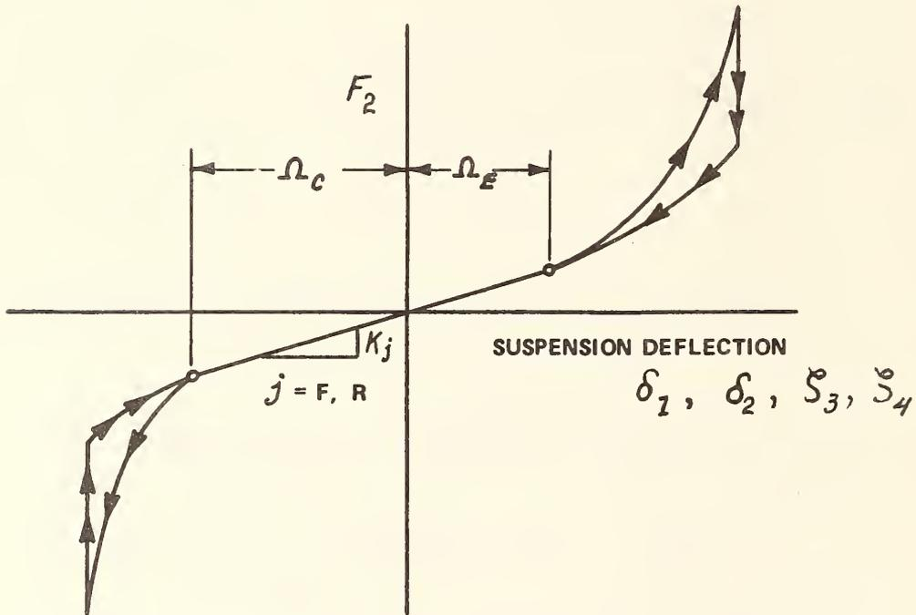
Figure 3.7 GENERAL FORM OF SIMULATED SUSPENSION LOAD-DEFLECTION CHARACTERISTICS (REFERENCE 2)
