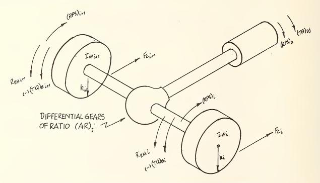
Figure 3.5 INERTIAL COUPLING OF DRIVE WHEELS
