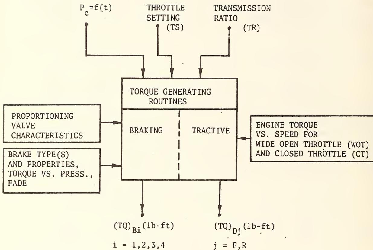
Figure 3.8 GENERATION OF WHEEL TORQUES
