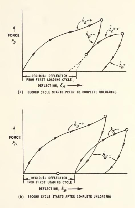
Figure 3,28 ASSUMED FORM OF LOAD-DEFLECTION FOR RECURRENT LOADING
