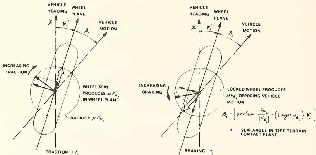
Figure 3.22<sup>1</sup> FRICTION CIRCLE CONCEPT
