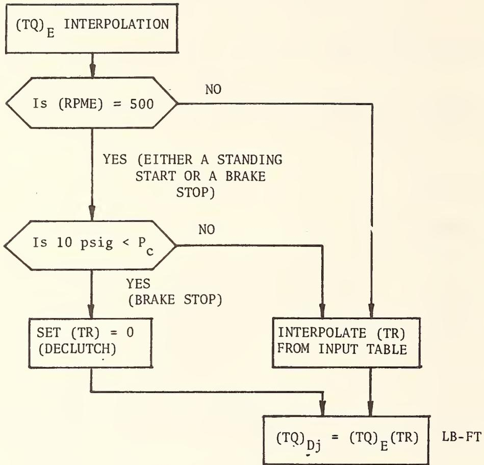
Figure 3.17 LOGIC TO PERMIT A STANDING START
