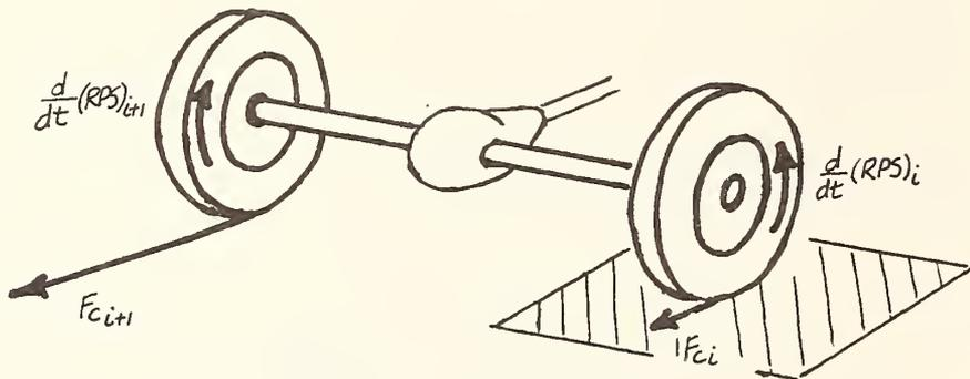
Figure 3.15 EFFECTS OF INERTIAL COUPLING OF DRIVE WHEELS
