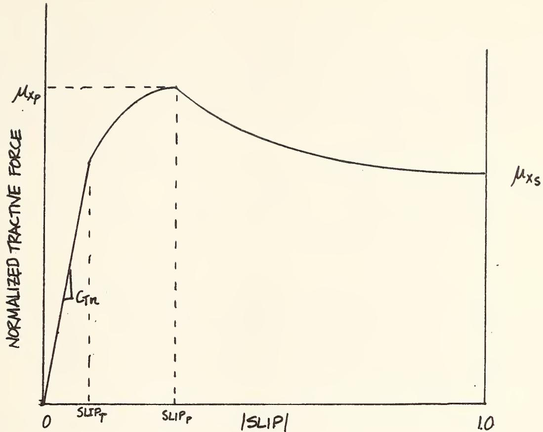
Figure 3.24 Normalized Tractive Force vs. SLIP Model
