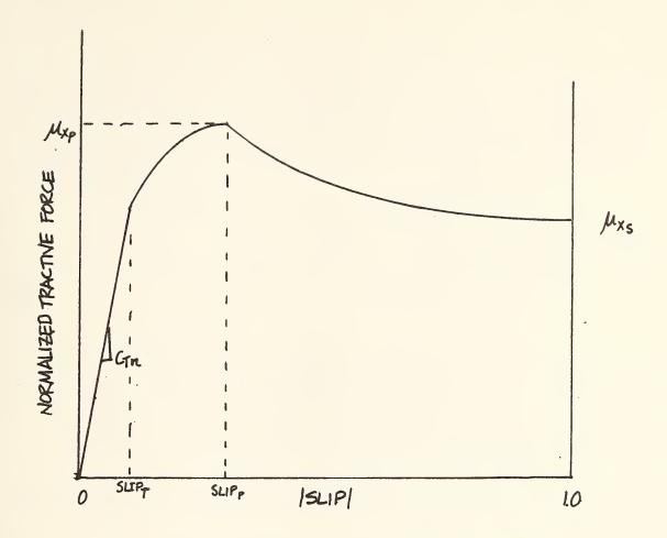
Figure 3,24 Normalized Tractive Force vs. SLIP Model
