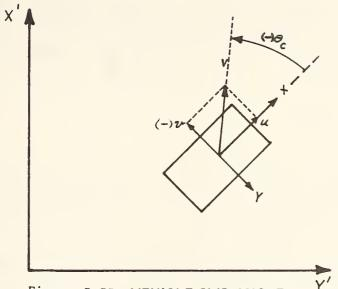
Figure 3.33 VEHICLE SLIP ANGLE
