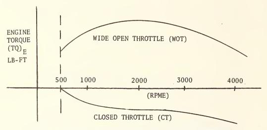
Figure 3.16 INPUTS TO DEFINE ENGINE PROPERTIES
