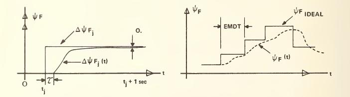
Figure 3.32 NEURO - MUSCULAR FILTER CHARACTERISTICS
