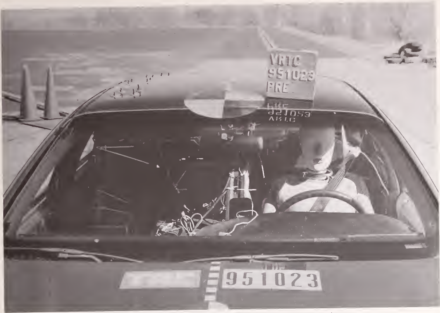
Figure A-12 Pre-Test Driver Dummy Frontal View
