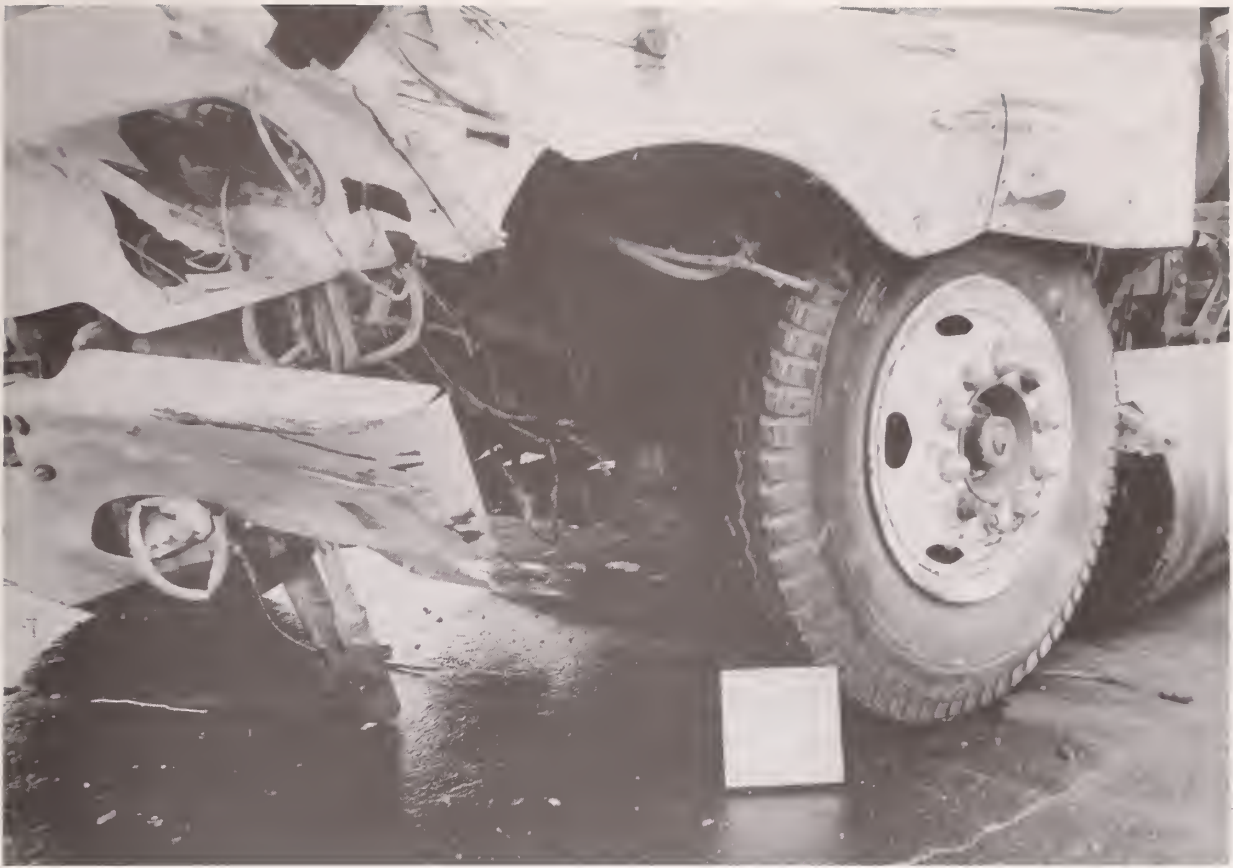
Figure A-31 Post-Test Heavy Truck Bumper - View 3
