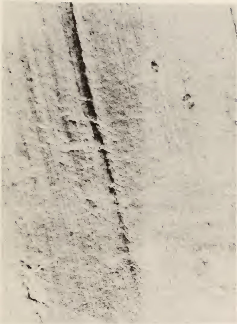
Figure 5-29 Crack growth striations nearer web surface - 49125X.
