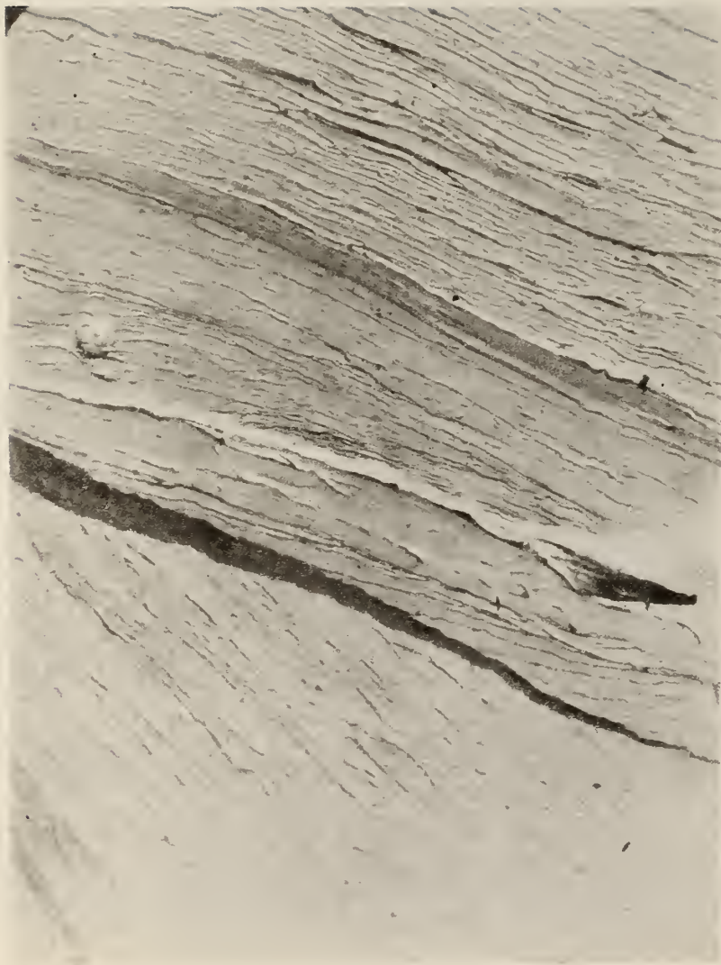
Figure 5-30 Cleavage in flange near bottom surface - 4300X.
