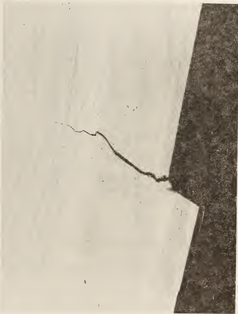
Figure 3-18 Typical failure at flange attachment with no transverse weld.
