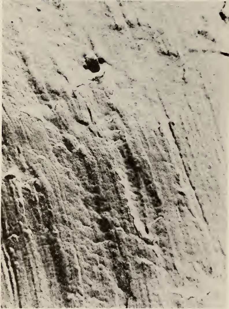
Figure 5-28 Crack growth striations nearest longitudinal stiffener - 49125X.
