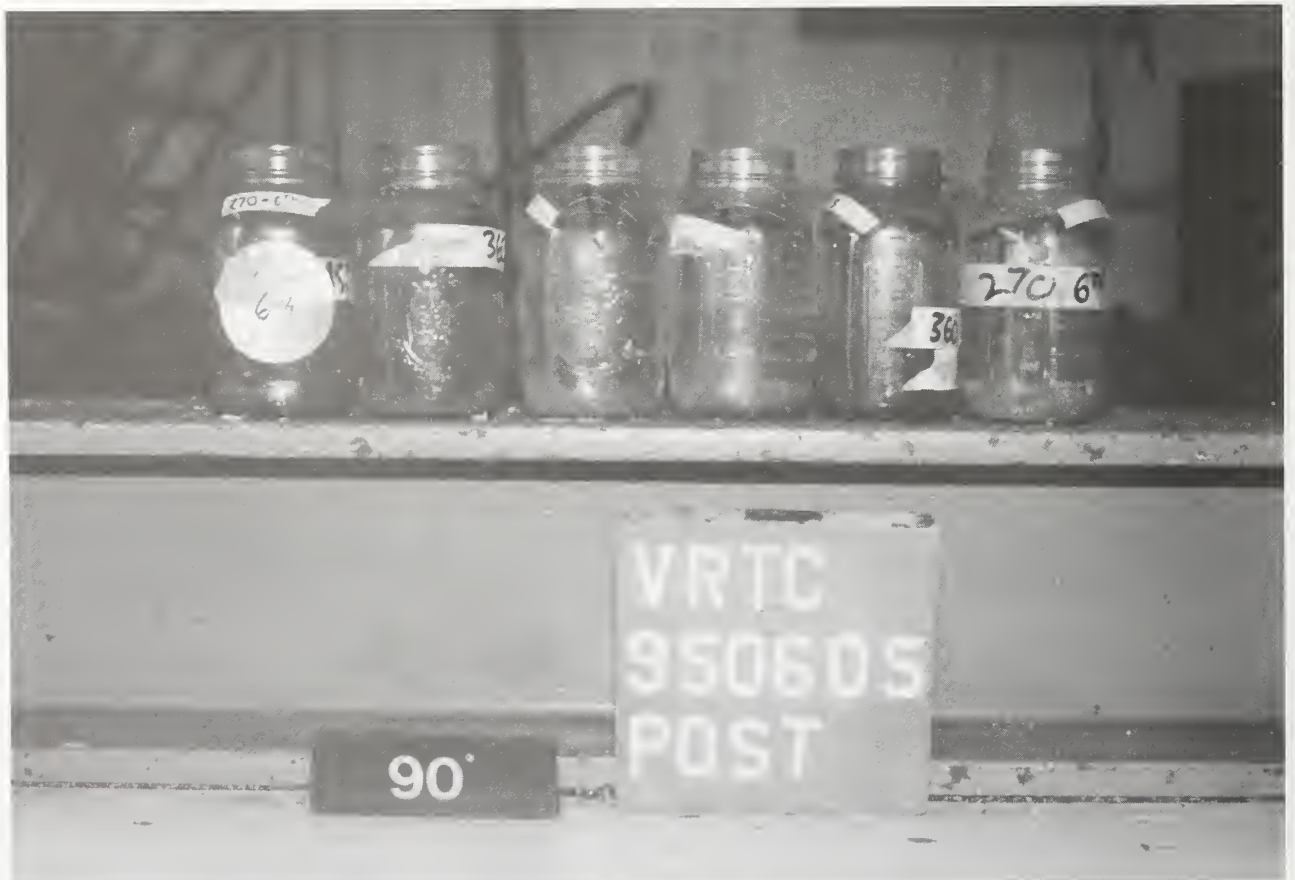
Figure A-48 Post-test Static Rollover Electrolyte Spillage 0° - 90°
