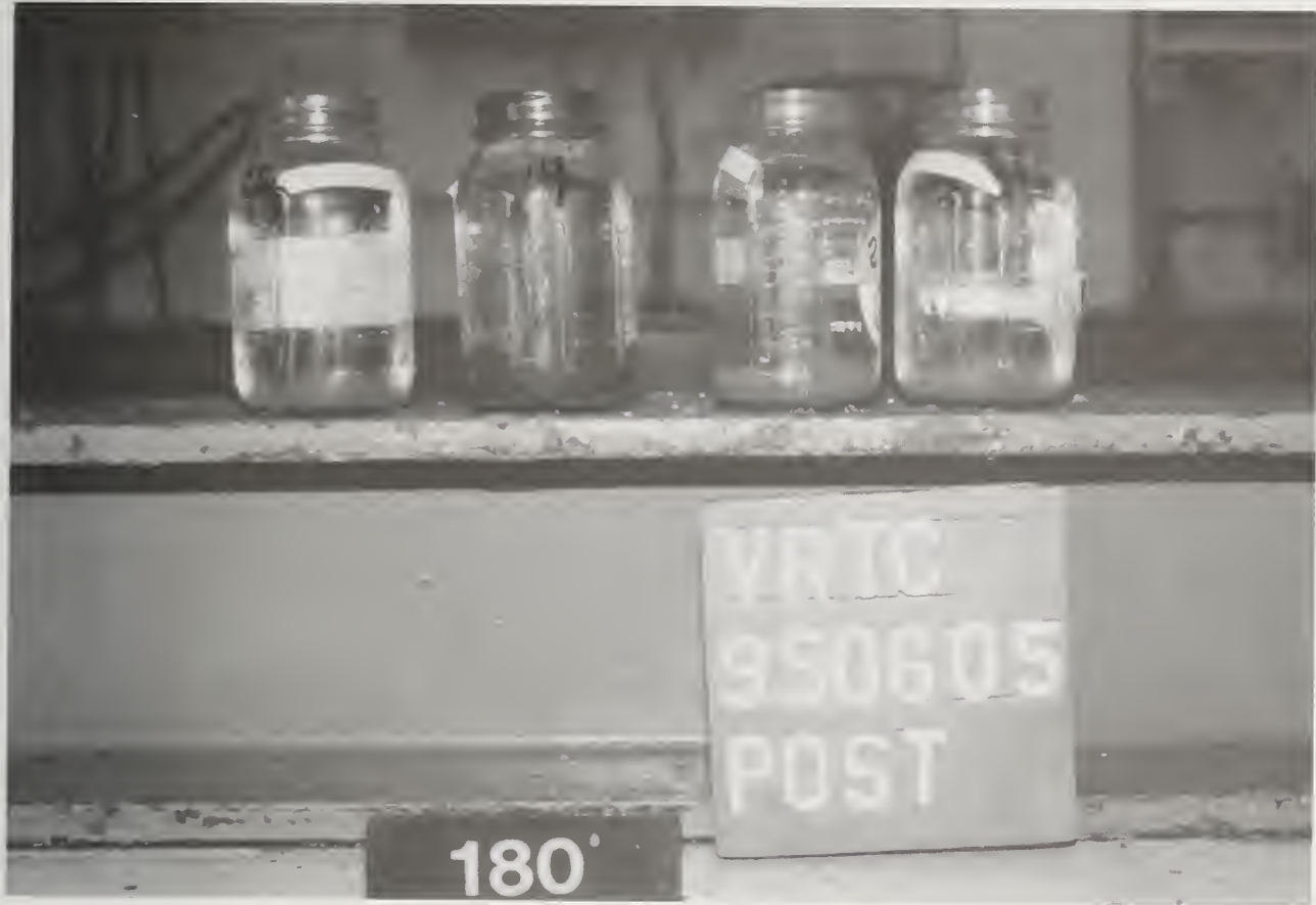
Figure A-49 Post-test Static Rollover Electrolyte Spillage 90° - 180°
