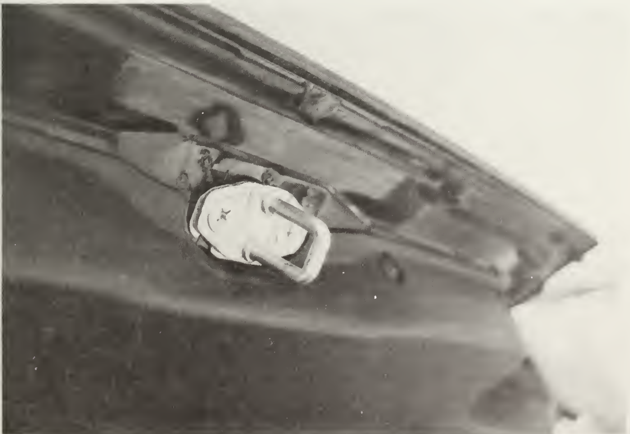
Figure A-18 Post-Test Rear Hatch Striker - View 1
