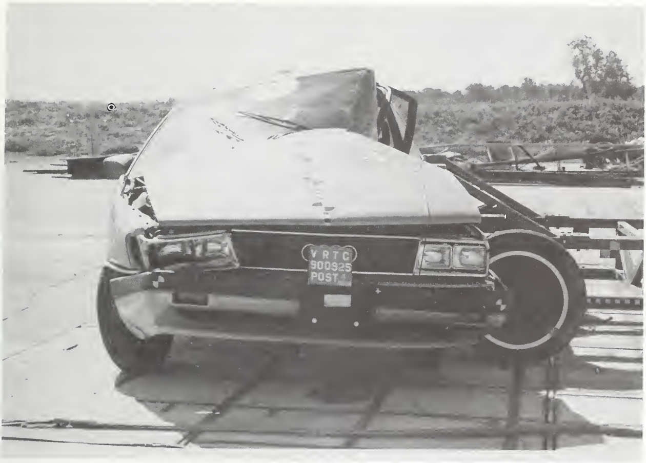
Figure A-36. POST-TEST OVERALL FRONT VIEW
