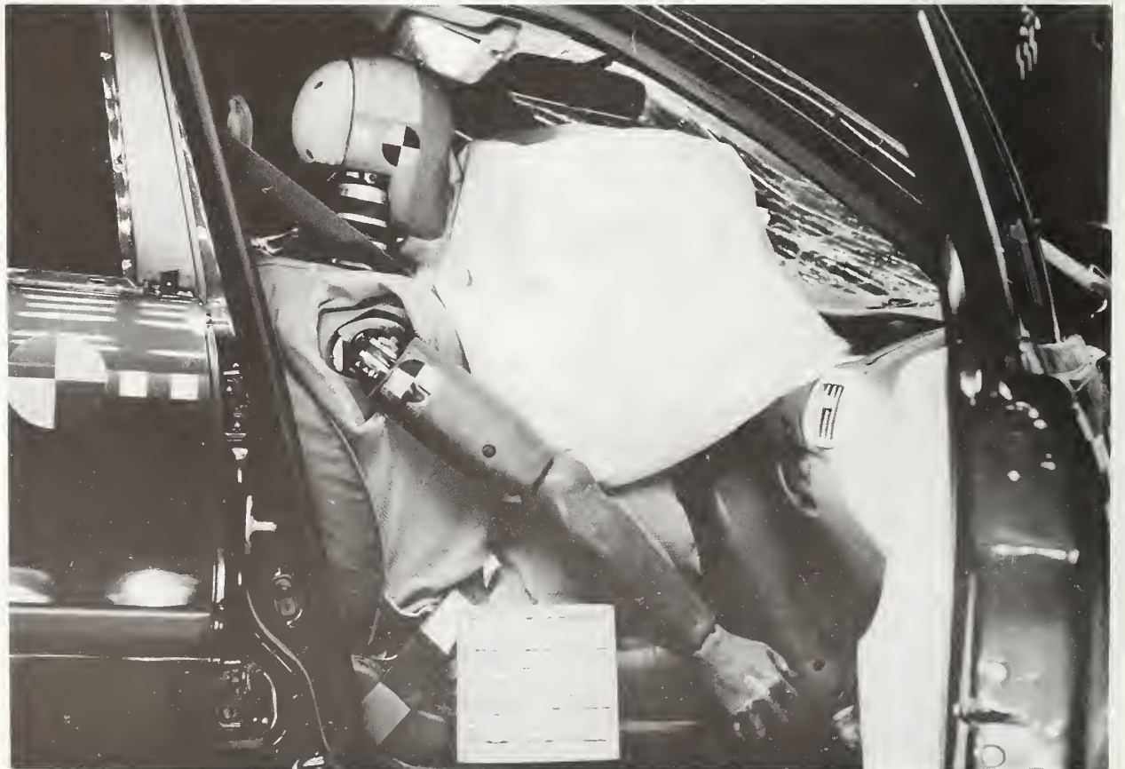
Figure A-30 Post-test Passenger Dummy and Vehicle Interior - View 1
