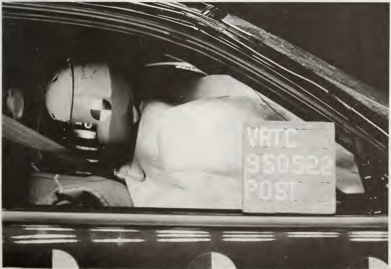
Figure A-24 Post-test Passenger Dummy Position View
