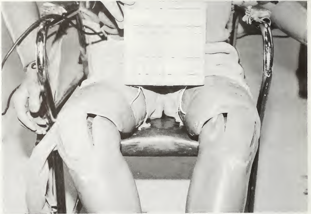
Figure A-37 Post-test Driver Dummy Knee Contact - View 1
