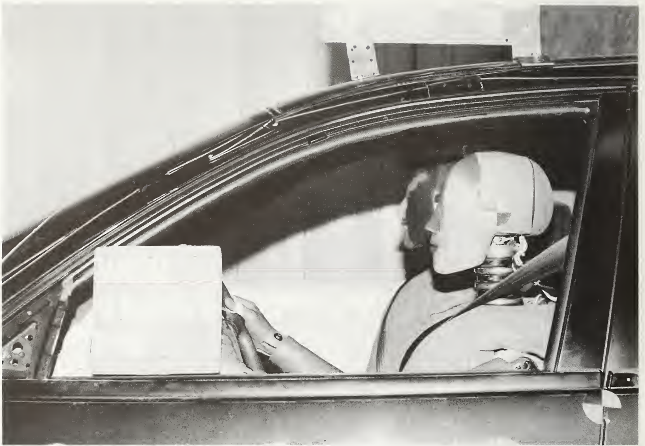
Figure A-22 Pre-test Driver Dummy Position View
