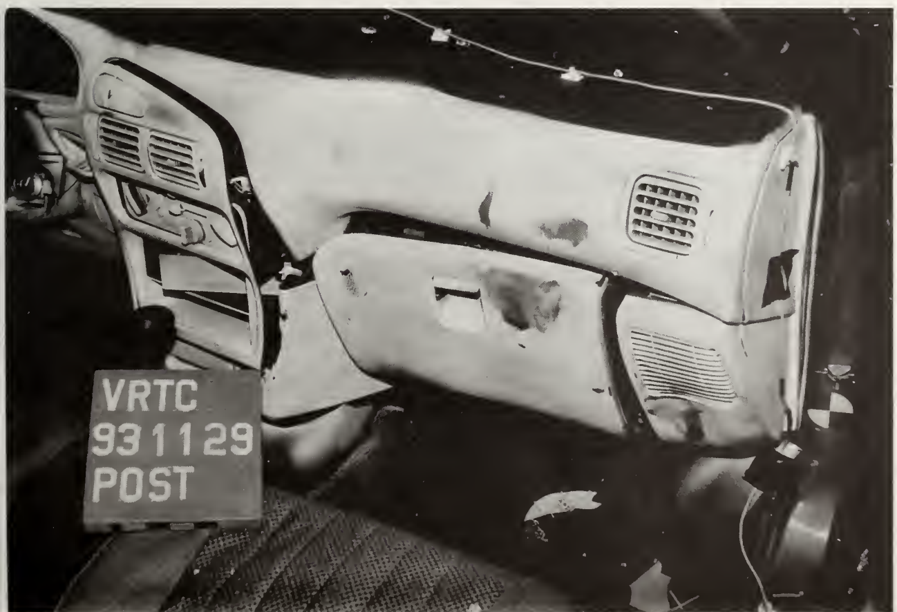
Figure A-42 POST-TEST PASSENGER DUMMY KNEE CONTACT - VIEW 2
