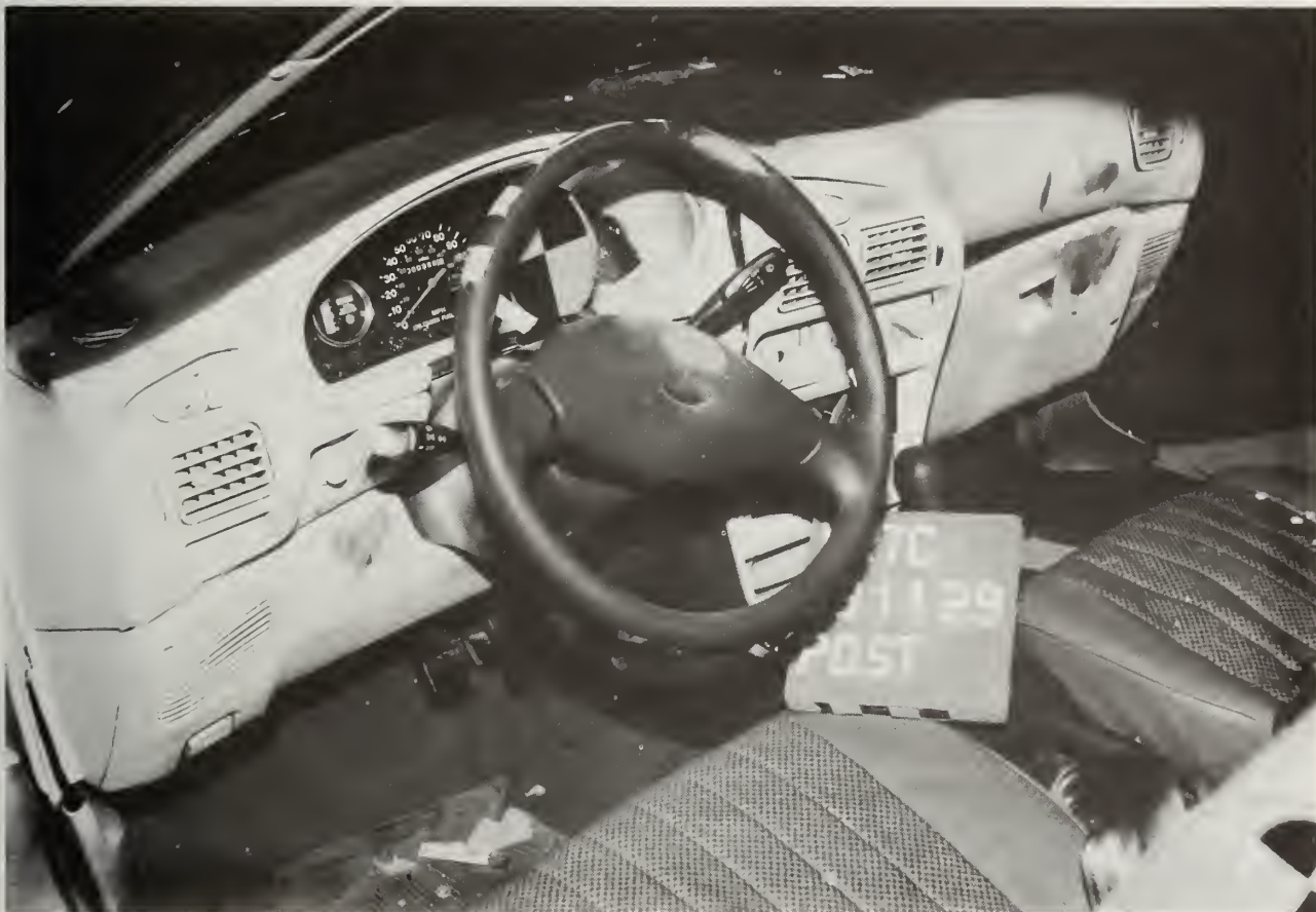
Figure A-37 POST-TEST DRIVER DUMMY HEAD CONTACT - VIEW 2
