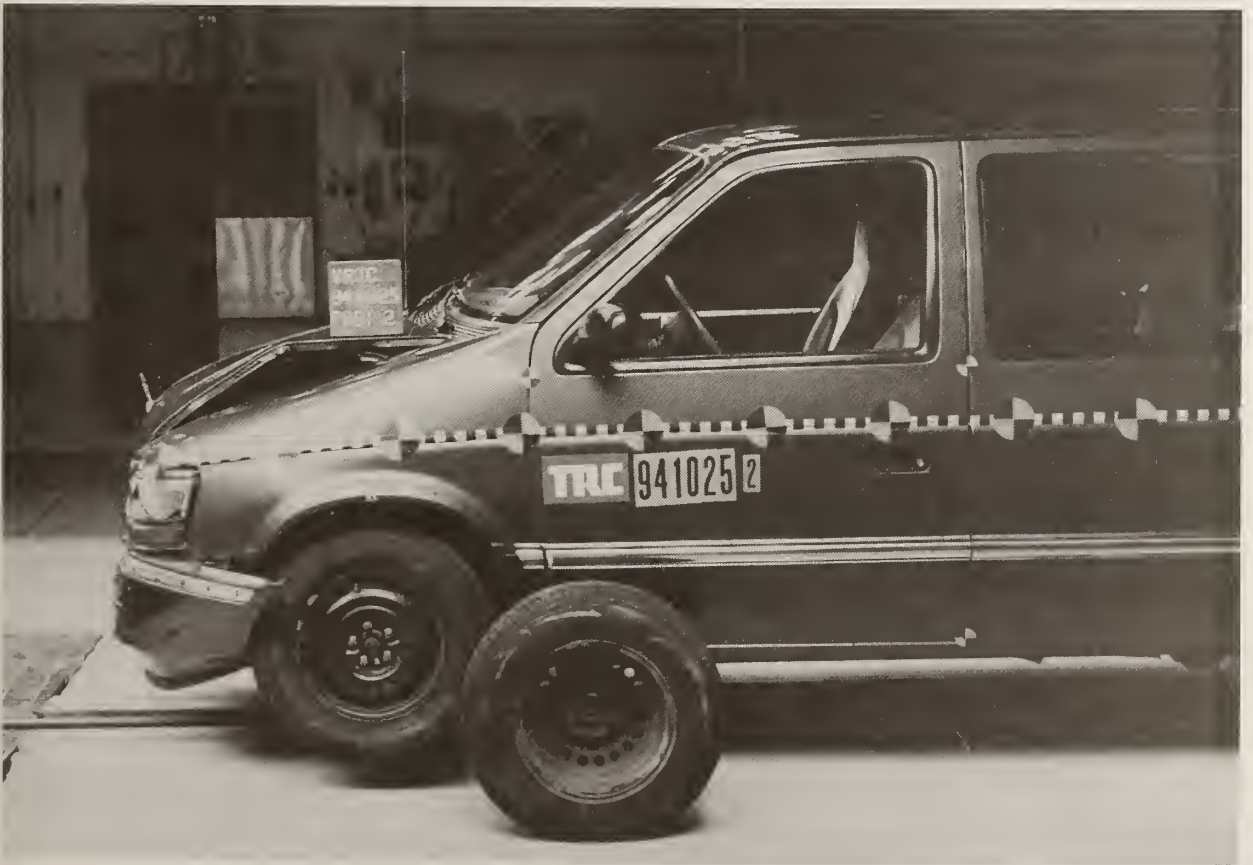
Figure A-13. Post-Test Left Side View
