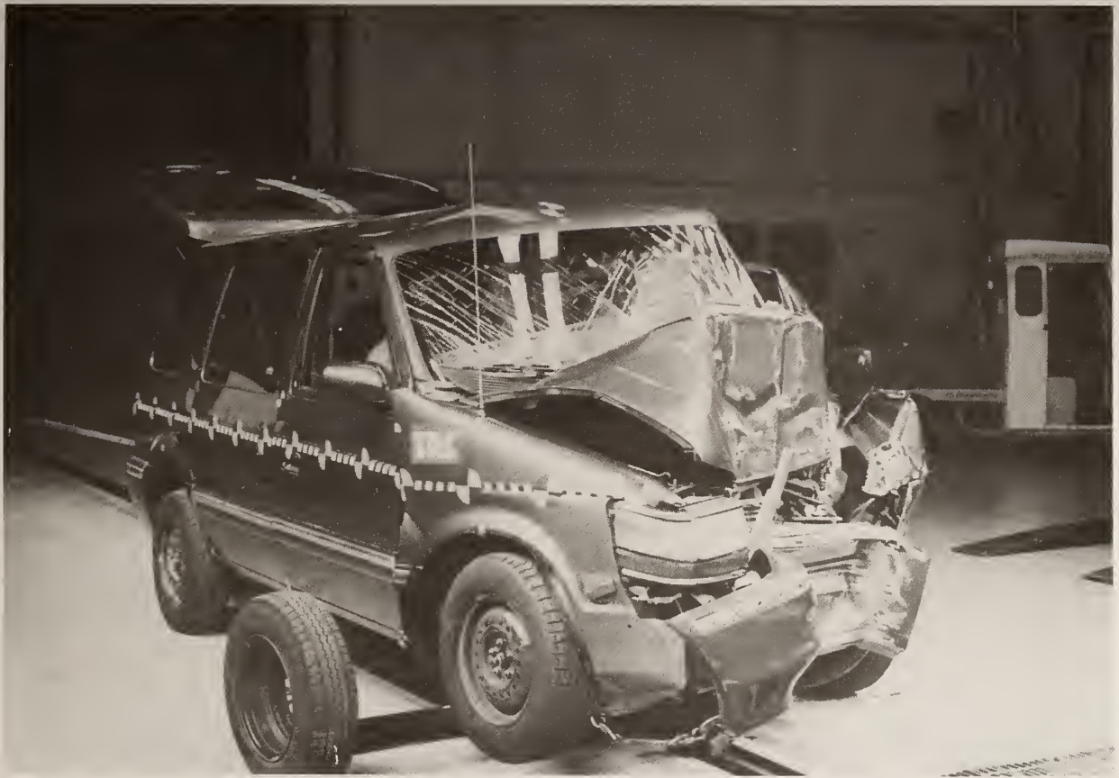
Figure A-34. Post-Test Right Front Three-Quarter View
