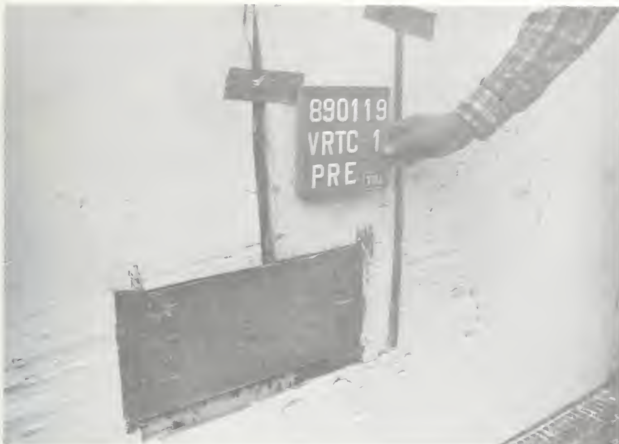
Figure A-9. PRE-TEST BARRIER CONTACT SWITCH
