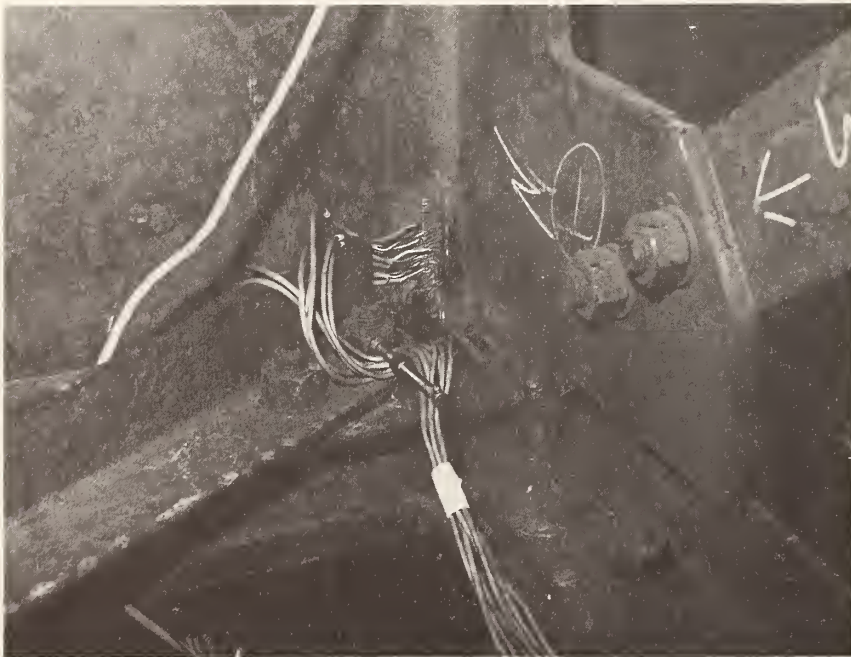
Fig. 63 Strips of Ten Strain Gages Mounted on North and South Faces of Web - Midspan - Assembly 4 - Girder 2
