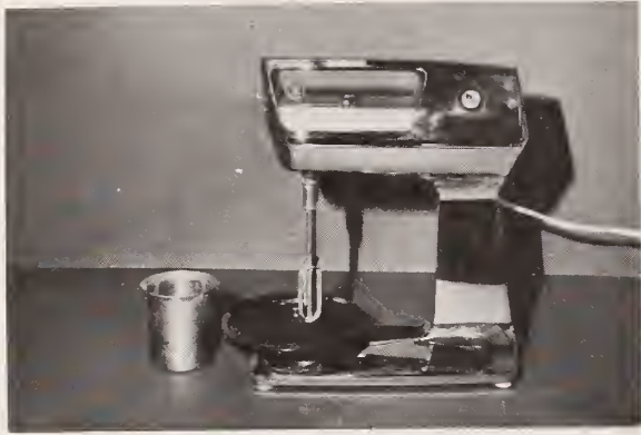
FIGURE 66A. MIXER USED FOR CEMENT PASTES
