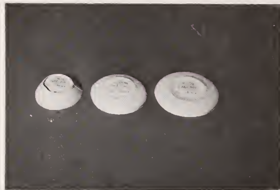
FIGURE 66C. PATS FORMED IN MINI-SLUMP TEST
