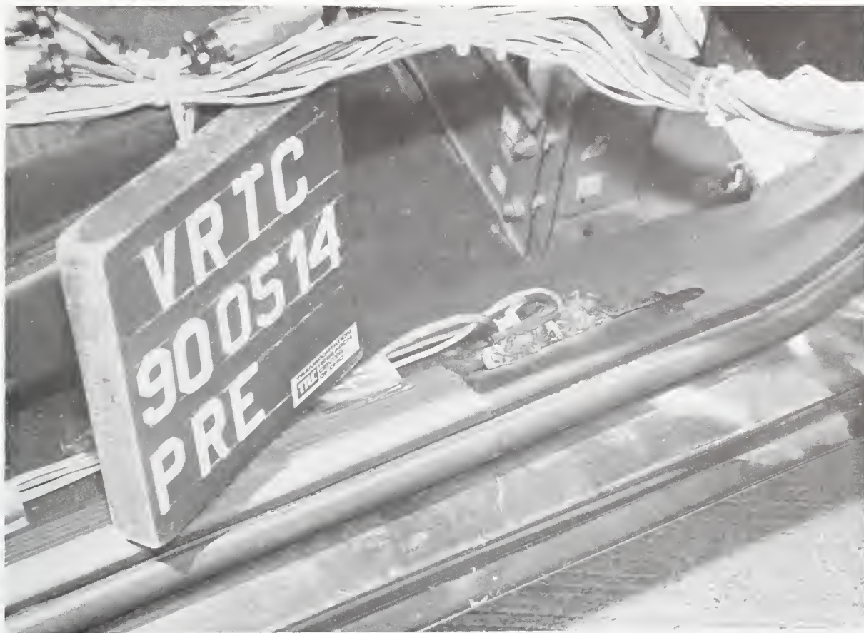
Figure A-21. PRE-TEST RIGHT FRONT SILL ACCELEROMETER VIEW
