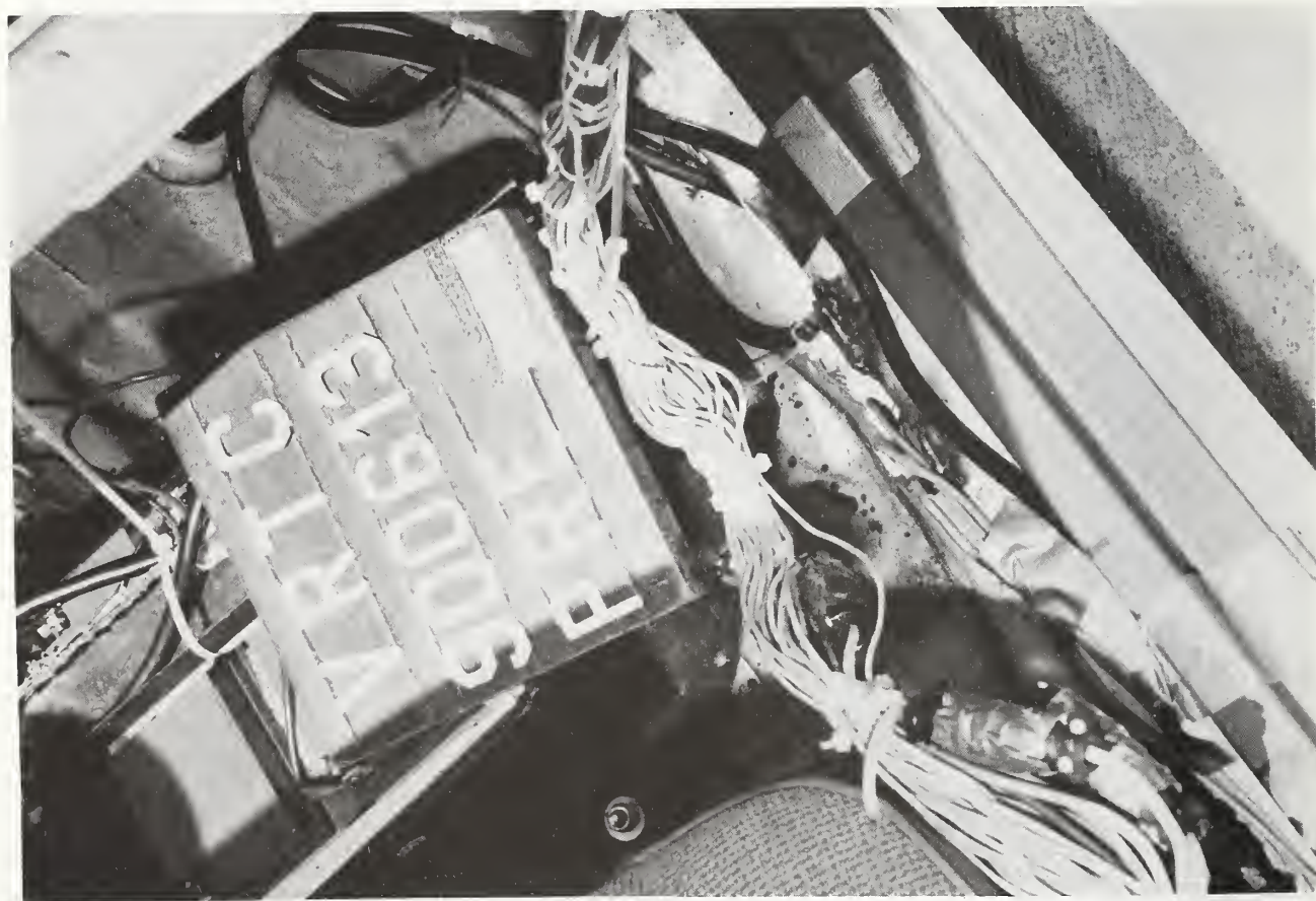
Figure A-24. PRE-TEST RIGHT FRONT SILL ACCELEROMETER VIEW
