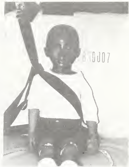
FIGURE 38. 83D007 Shoulder Belt With Adjustment Strap, Pre-Test
