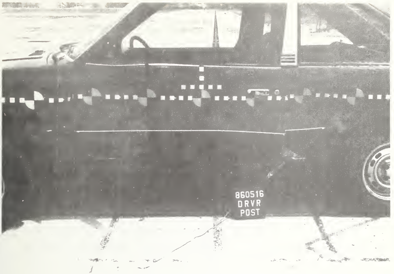
Figure A-15. POST-TEST FRONT DRIVER DOOR VIEW
