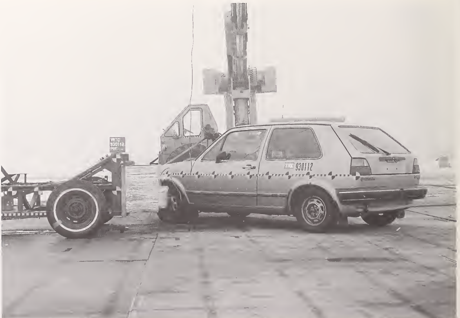
Figure A-8. PRE-TEST IMPACTOR FACE & VEHICLE ALIGNMENT - VIEW 2
