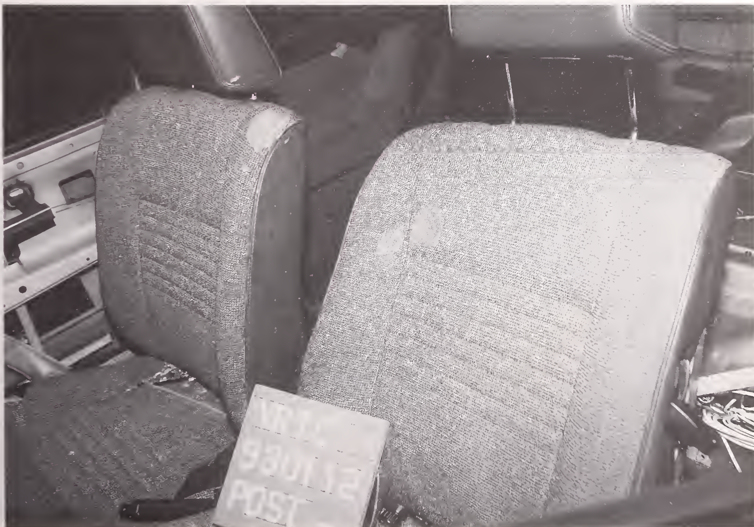
Figure A-26. POST-TEST DRIVER DUMMY HEAD CONTACT - VIEW 2
