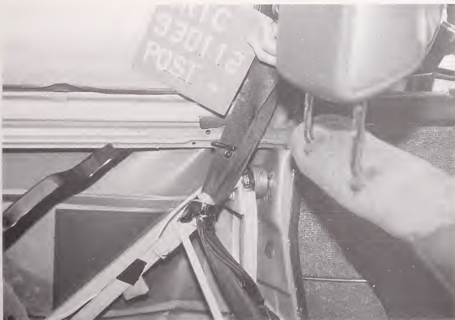
Figure A-14. POST-TEST DOOR LATCH LOAD CELL - VIEW 2
