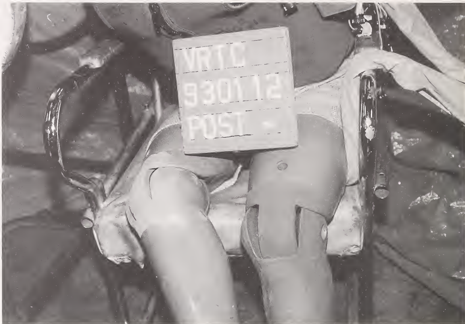
Figure A-27. POST-TEST DRIVER DUMMY KNEE CONTACT - VIEW 1
