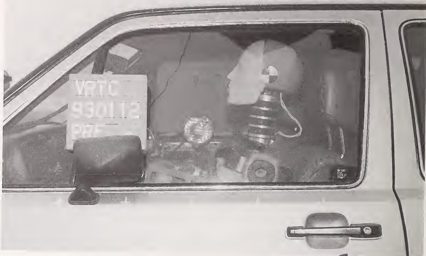
Figure A-15. PRE-TEST DRIVER DUMMY POSITION - VIEW 1
