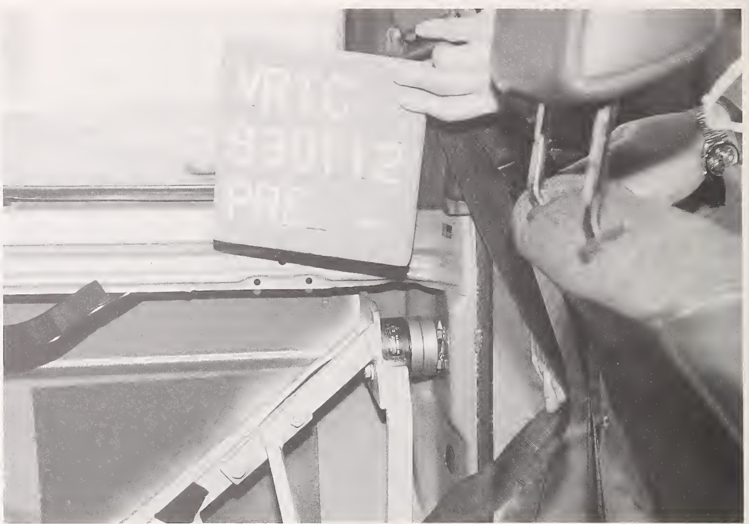
Figure A-11. PRE-TEST DOOR LATCH LOAD CELL - VIEW 2
