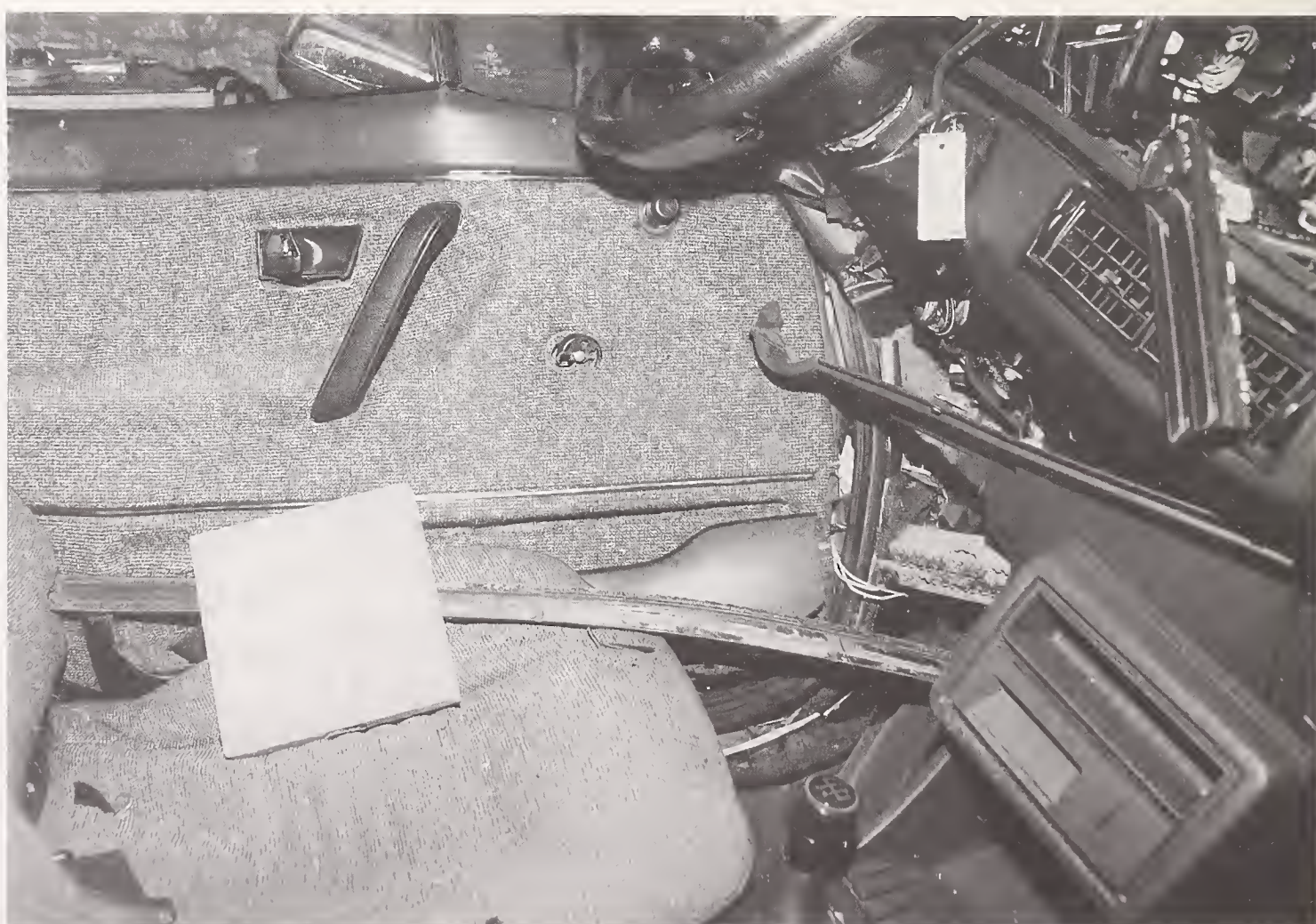
Figure A-28. POST-TEST DRIVER DUMMY KNEE CONTACT - VIEW 2
