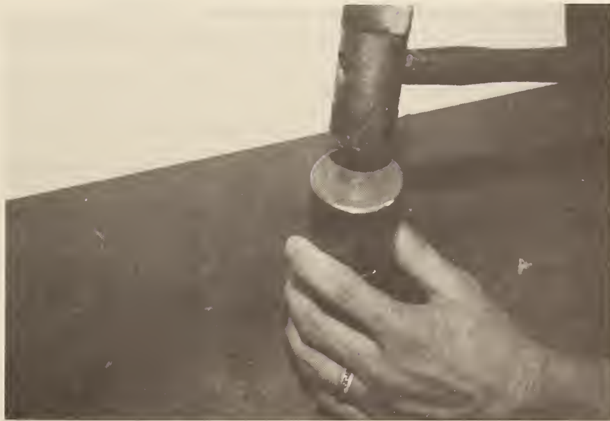
Fig. A-21. Top of die is put in place.
