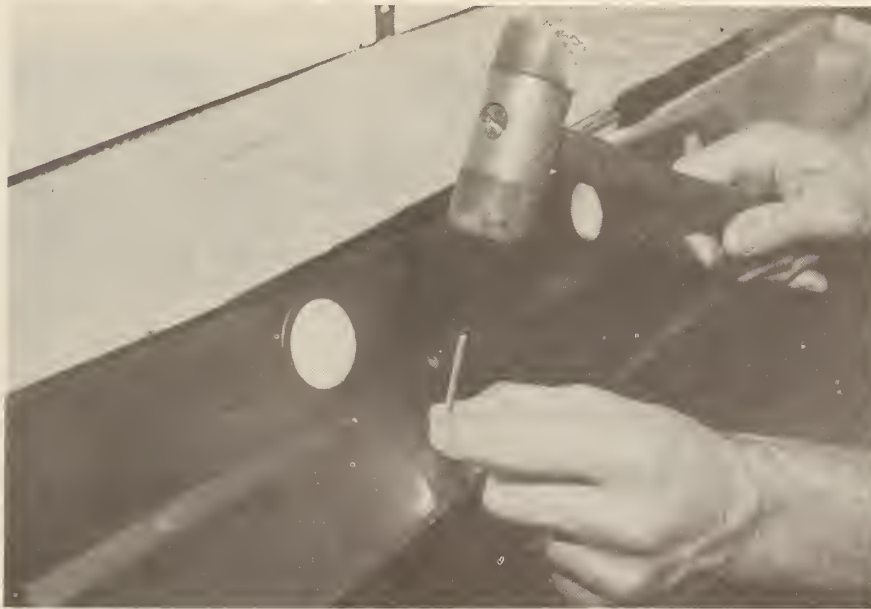
Fig. A-14. Diaphragm replacement : Remove press ring by carefully driving a small punch through three holes on the back of the blade.
