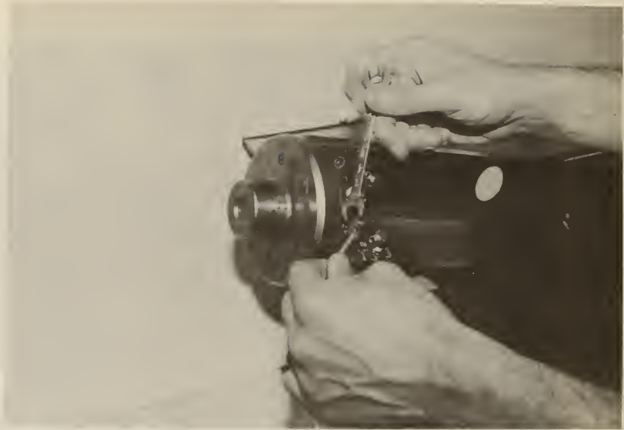
Fig. A-7. If not previously done, connect numbered lines to appropriately numbered elbows on the vane.
