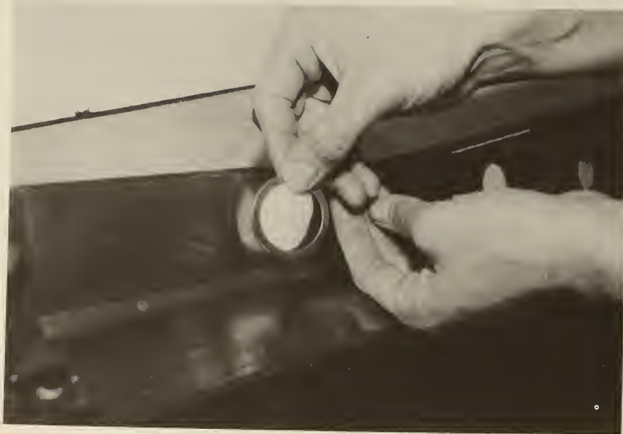
Fig. A-15. Hold a new diaphragm and the press ring in place. The ring is pushed down with a special C-clamp (not shown).
