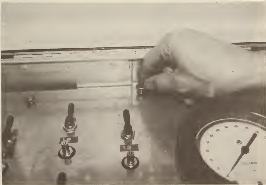
Fig. A-1. Assembly : Console pressure regulator is turned counterclockwise so knob is loose, so no pressure will be applied during hook-ups.
