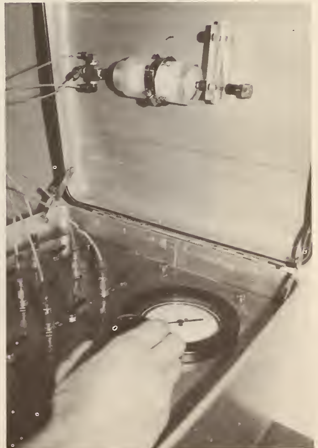
Fig. A-9. Measurement : Toggle valve is opened to transmit gas pressure to a pressure cell.
