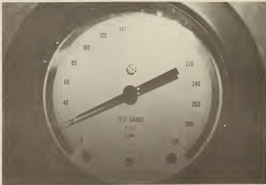
Fig. A-12. The pressure gauge is immediately read and the reading recorded.
