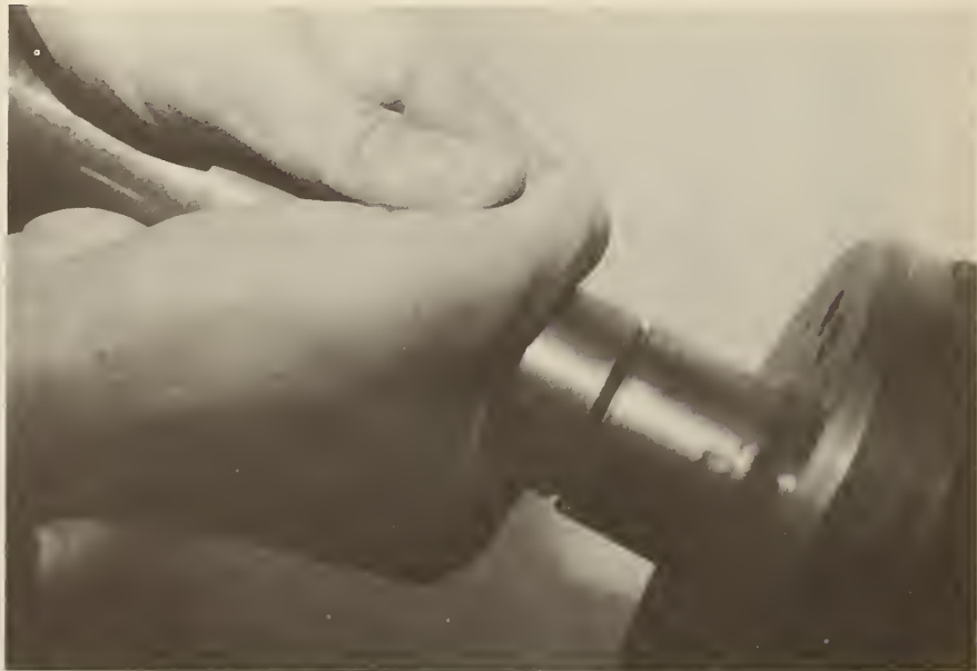
Fig. A-8. Vane is fastened to an special connector which allows drill rod weight to be lifted off the vane. Assembly is then attached to any conventional rotary exploration drilling machine.
