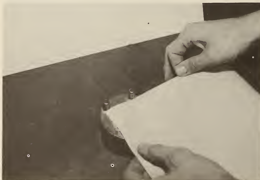
Fig. A-16. Diaphragm manufacture : Teflon sheet is laid on the punch anvil.
