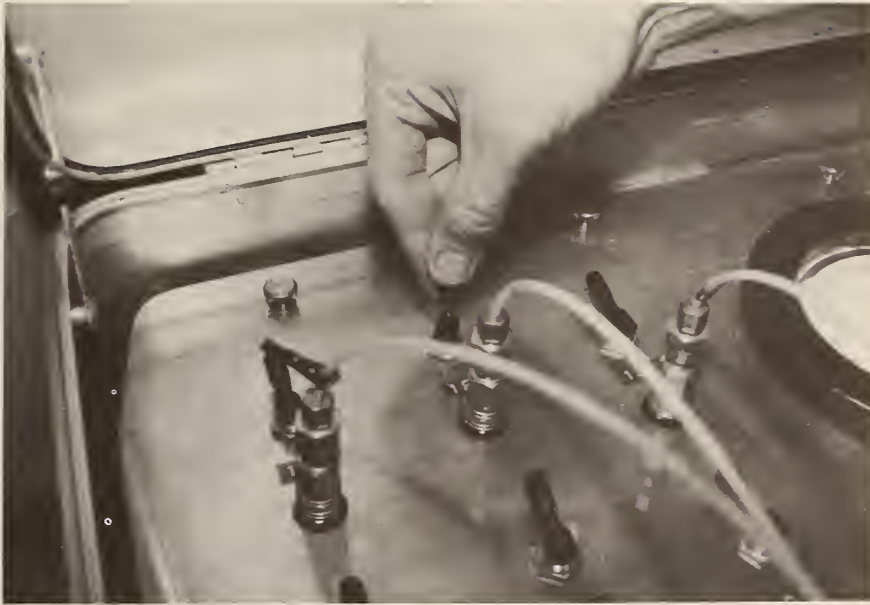
Fig. A-9. Measurement : Toggle valve is opened to transmit gas pressure to a pressure cell.
