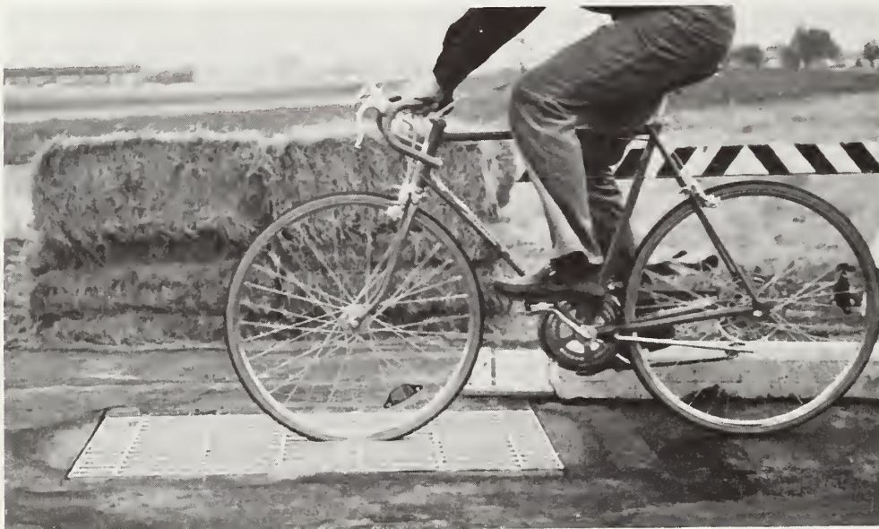
Figure 3-4. - Severe tire deformation on a grate with 8 in (203 mm) transverse bar spacing. Photo H-1765-59
