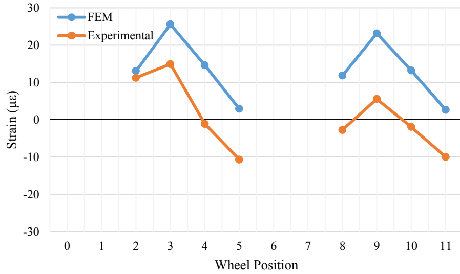
Figure C-3: FEM vs. Experimental comparison of strain gage 2L for Blanchette Bridge test
