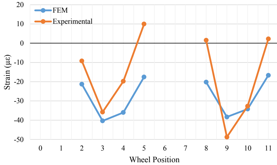
Figure C-7: FEM vs. Experimental comparison of strain gage 4 for Blanchette Bridge test
