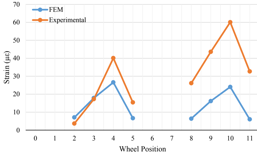
Figure C-11: FEM vs. Experimental comparison of strain gage 8L for Blanchette Bridge test
