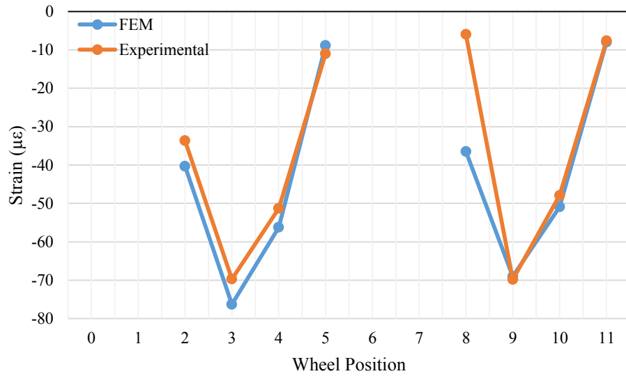
Figure C-7: FEM vs. Experimental comparison of strain gage 4 for Blanchette Bridge test
