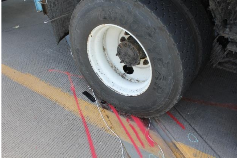
Figure 6-14: Wheel position locations of static test for front rear tire
