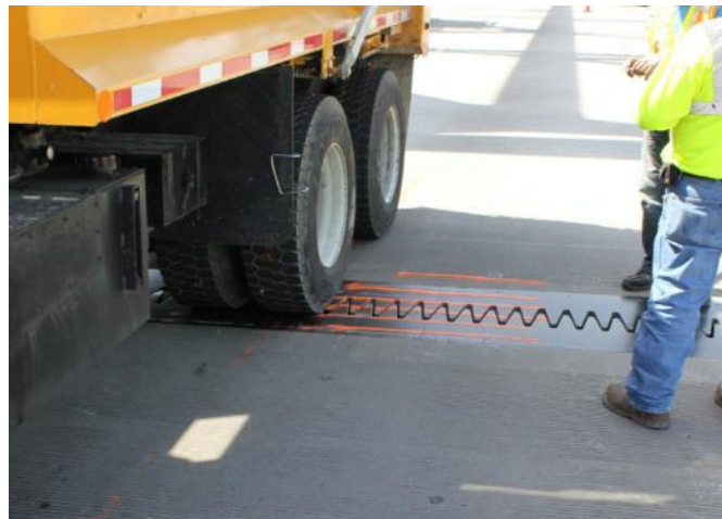
Figure 6-8: Wheel position locations during static test for front rear tire
