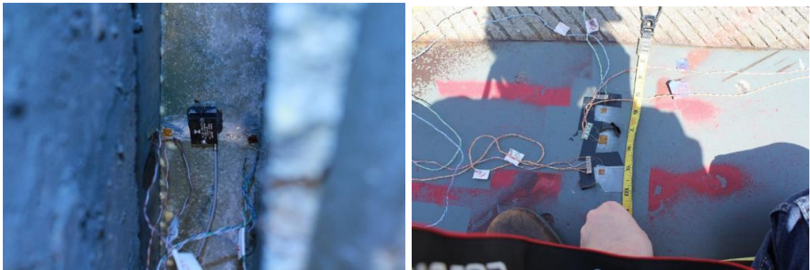
Figure 6-15: Strain gage arrangement attached to sliding plate
