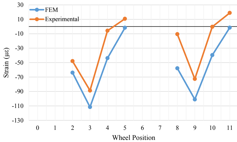
Figure C-3: FEM vs. Experimental comparison of strain gage 2L for Blanchette Bridge test
