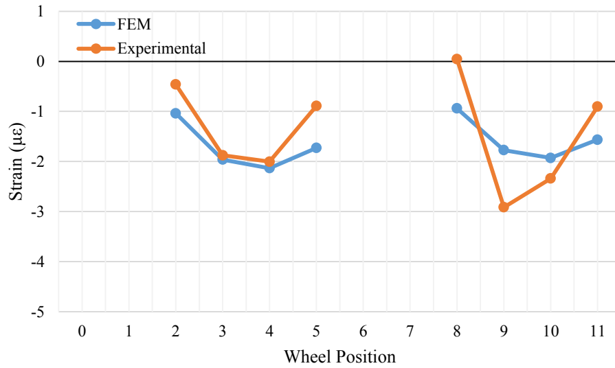
Figure C-9: FEM vs. Experimental comparison of strain gage 6 for Blanchette Bridge test
