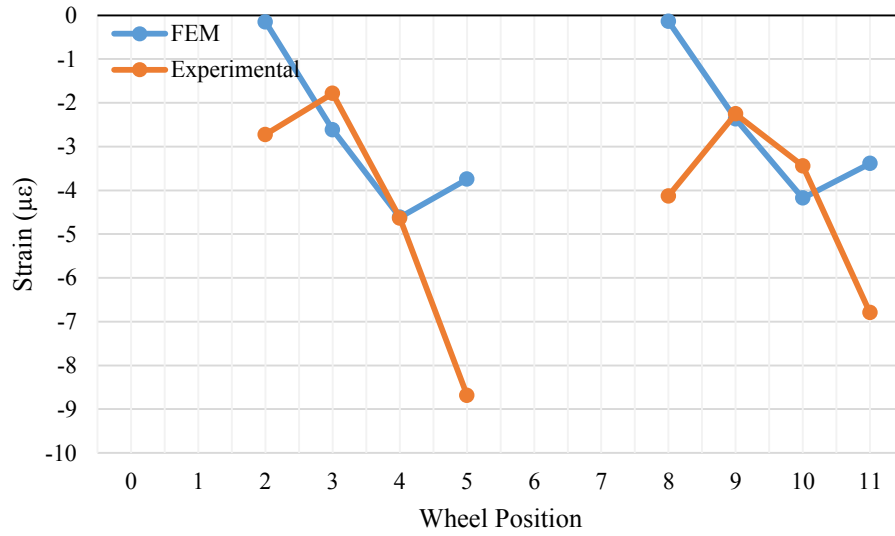
Figure C-9: FEM vs. Experimental comparison of strain gage 6 for Blanchette Bridge test
