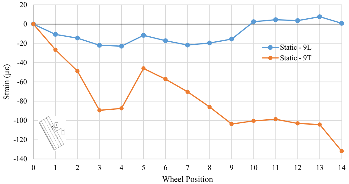
Figure B-25: Static data for strain gage 9 from Route 350 over I-435 bridge test
