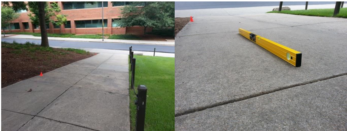
Figure 19. Initial Grade Field Data Test Location and SmartTool™ Digital Level
