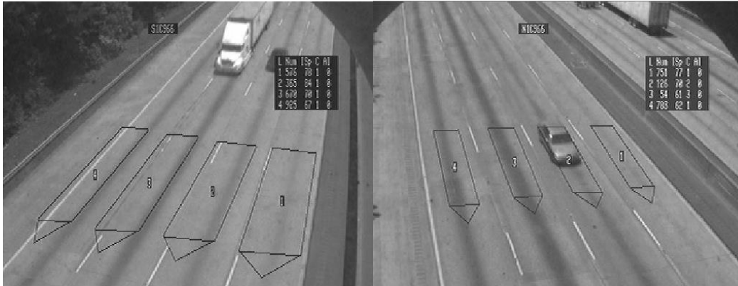
Figure 12: First Round, Gantry-mounted VDS Camera Views (Left: Southbound Station 285-1053; Right: Northbound Station 285-0210)
