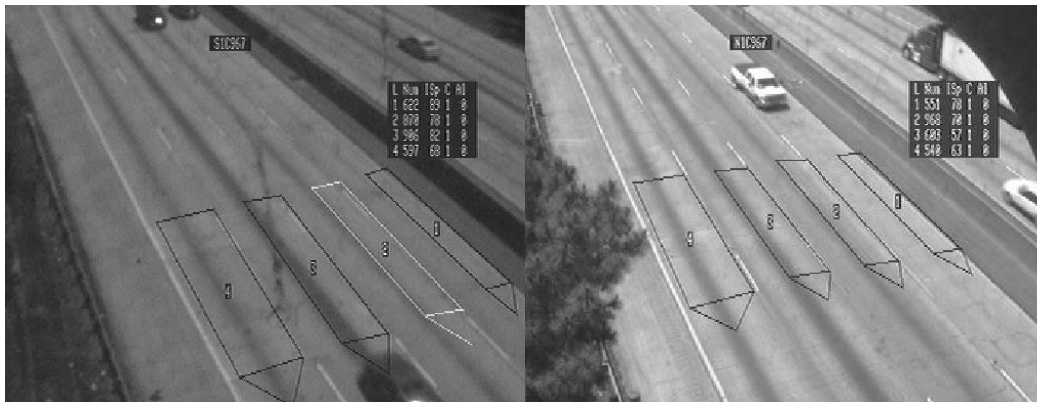
Figure 8: First Round, Pole-mounted VDS Camera Views (Left: Southbound Station 285-1052; Right: Northbound Station 285-0211)
