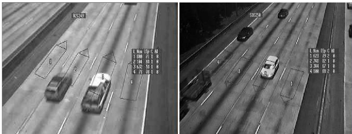
Figure 19: Camera Views for VDS Units on I-285 near US-78 (Left: Northbound Station 285-1980; Right: Southbound Station 285-0065)
