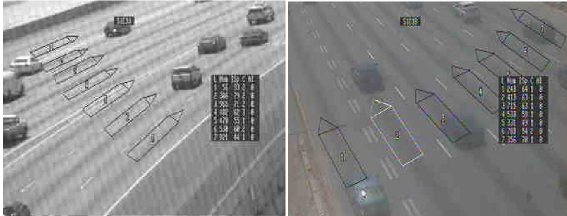
Figure 30: Camera Views for VDS Units on I-75/85 Connector (Left: 14 th St. Camera, Station 10131; Right: 10 th Street Camera, Station 10132)
