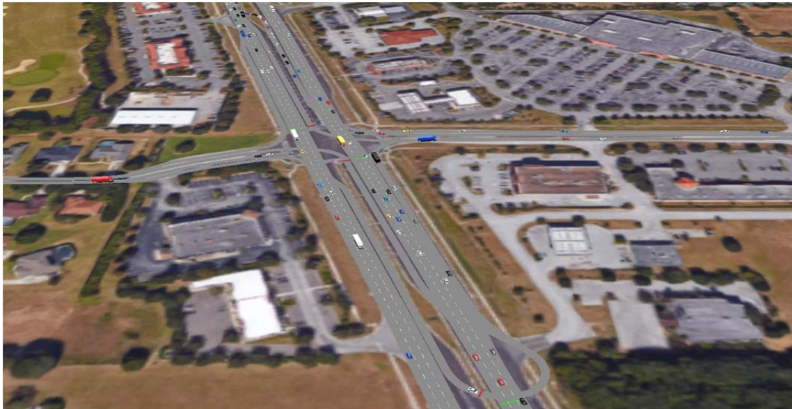
Figure 70: RCUT Intersection Coded in VISSIM
