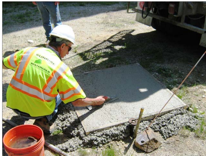
Figure 6 Preparing the trial batch sample
