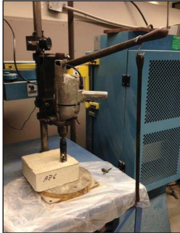
Figure 8 Drill press used to create powder samples
