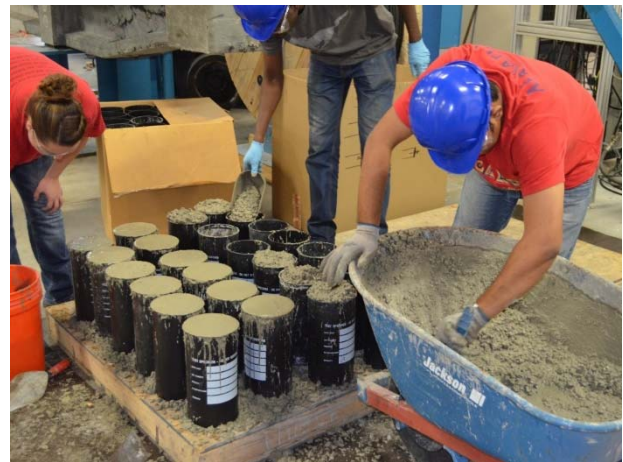
Figure 3.43: Preparation of concrete cylinders
