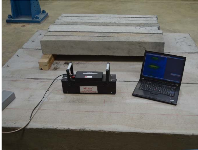
Figure 3.53: Ultrasonic assessment set-up for S2-1.
