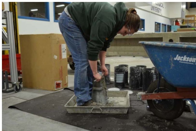
Fig. 3.23: Slump Test / Cylinders Preparation
