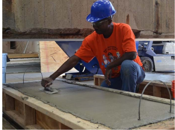
Fig. 3.41: Leveling top of specimen 2 beams
