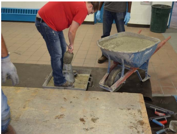
Figure 3.42: Checking for slump
