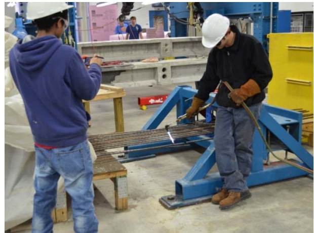
Figure 3.25: Releasing of steel strands.
