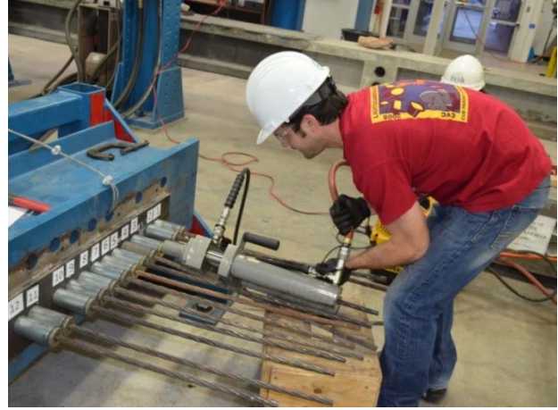
Figure 3.21: Prestressing steel strands
