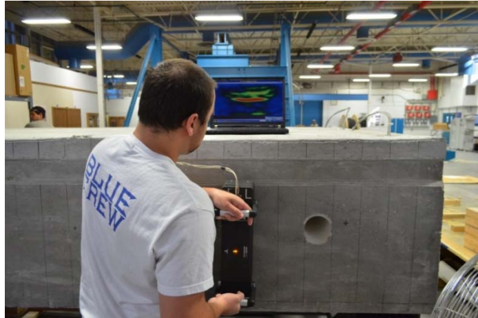
Figure 3.28: Scanning on the side of S1-1
