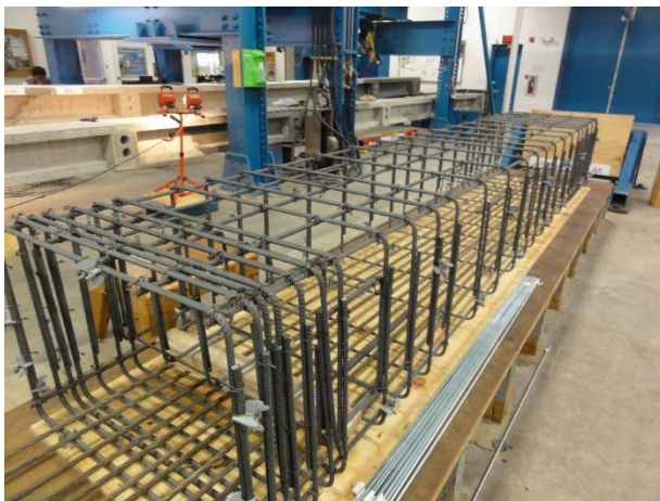
Figure 3.11: Reinforcement cages for box-beam
