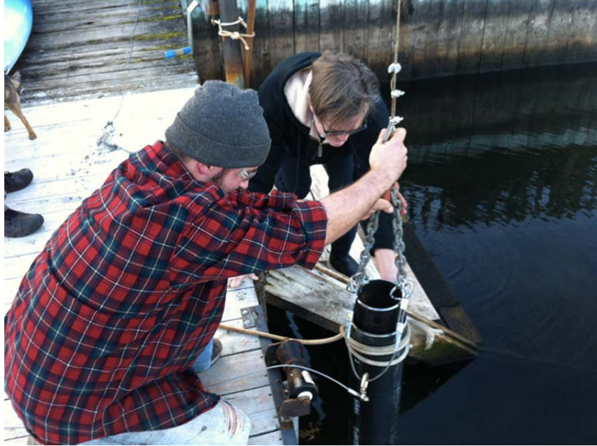
Figure 8: A subscale pile being prepared for testing
