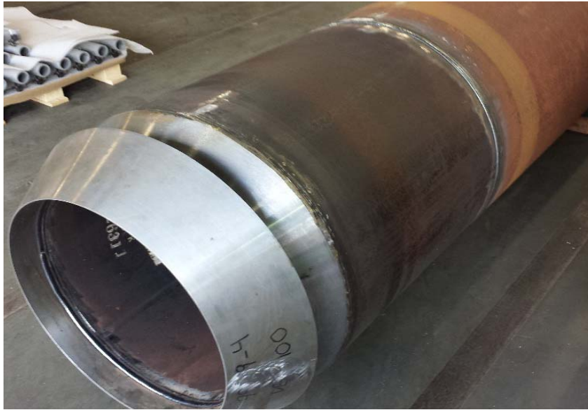
Figure 15: Double pile stem as delivered to Orion Marine
