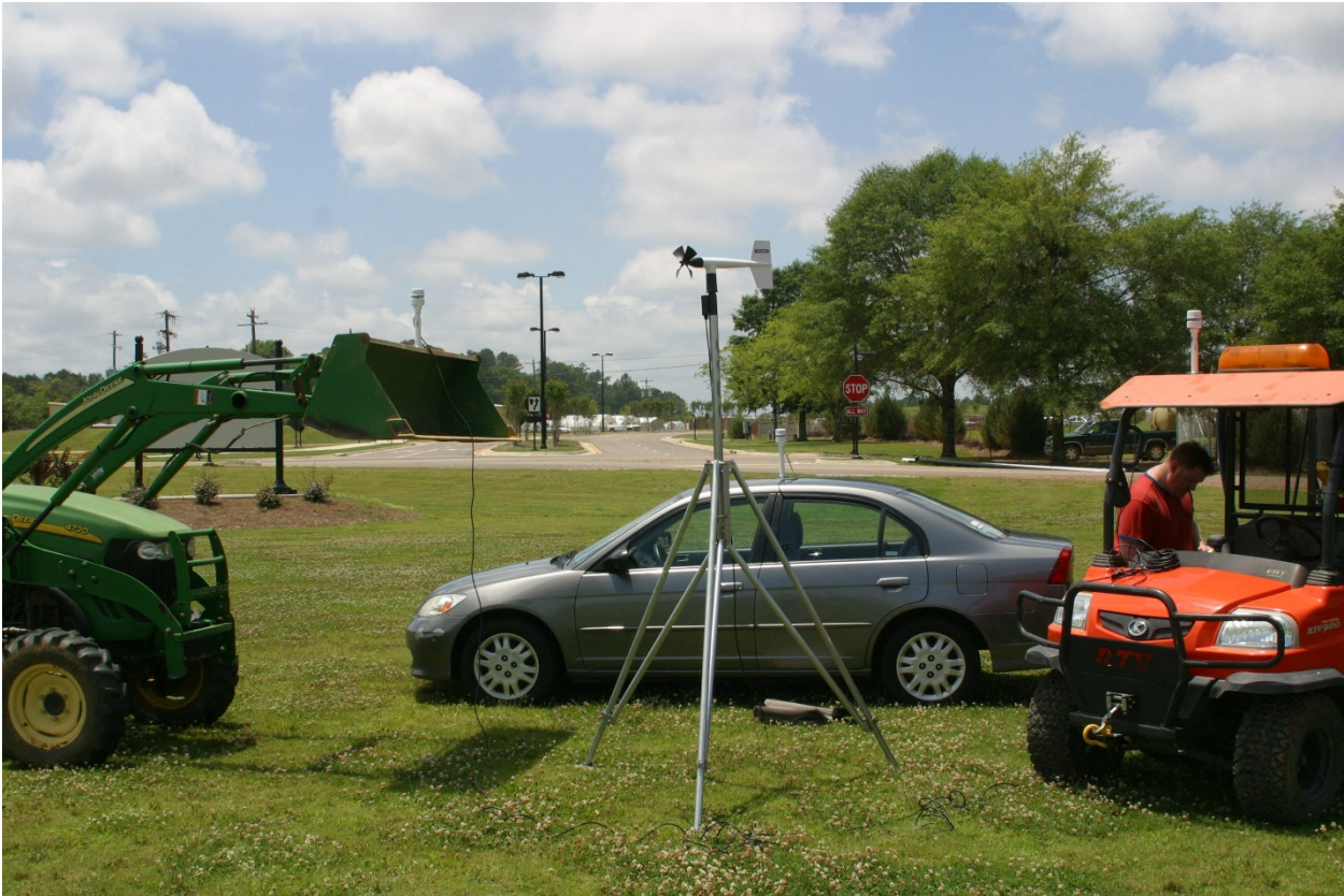
Figures 1, 2, 3. Initial stationary testing of Watchdog Sprayer Station and Young anemometer, June 3, July 16, and August 3, 2014, respectively, at the Rodney R. Foil Plant Science Research Center.
